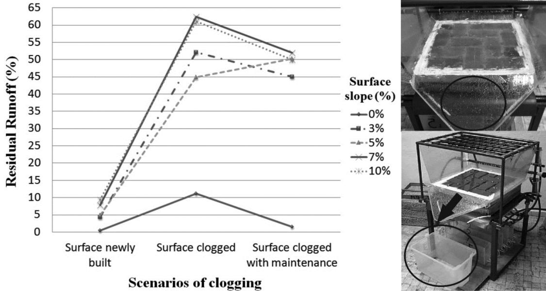
**Figure 3. Infiltration capacity of the ICBP surface in terms of its residual runoff depending on the surface slope and the scenario of clogging.**
