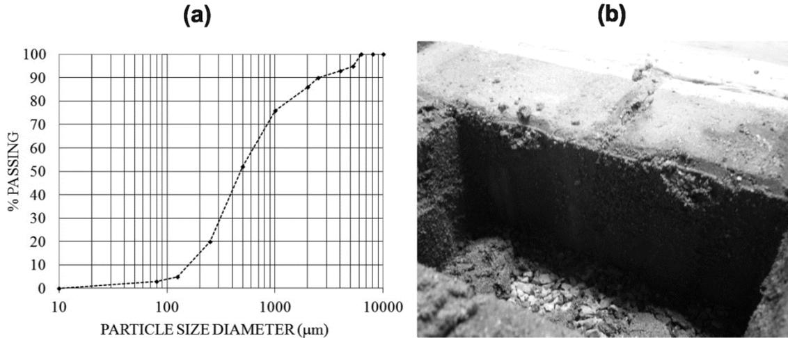
**Figure 2. (a) Particle size diameter distribution of the sediments used to clog the ICBP surface. (b) Sediments clogging the slots between blocks in the clogged surface scenario.**
