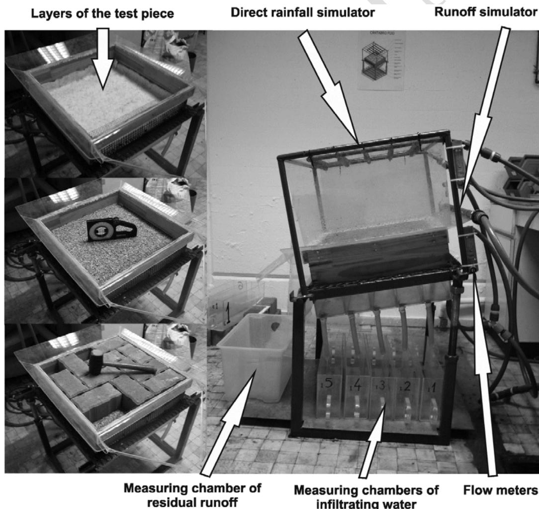
**Figure 1. Scheme of the improved CF Infiltrometer of the University of Cantabria with the layers of the test piece.**
