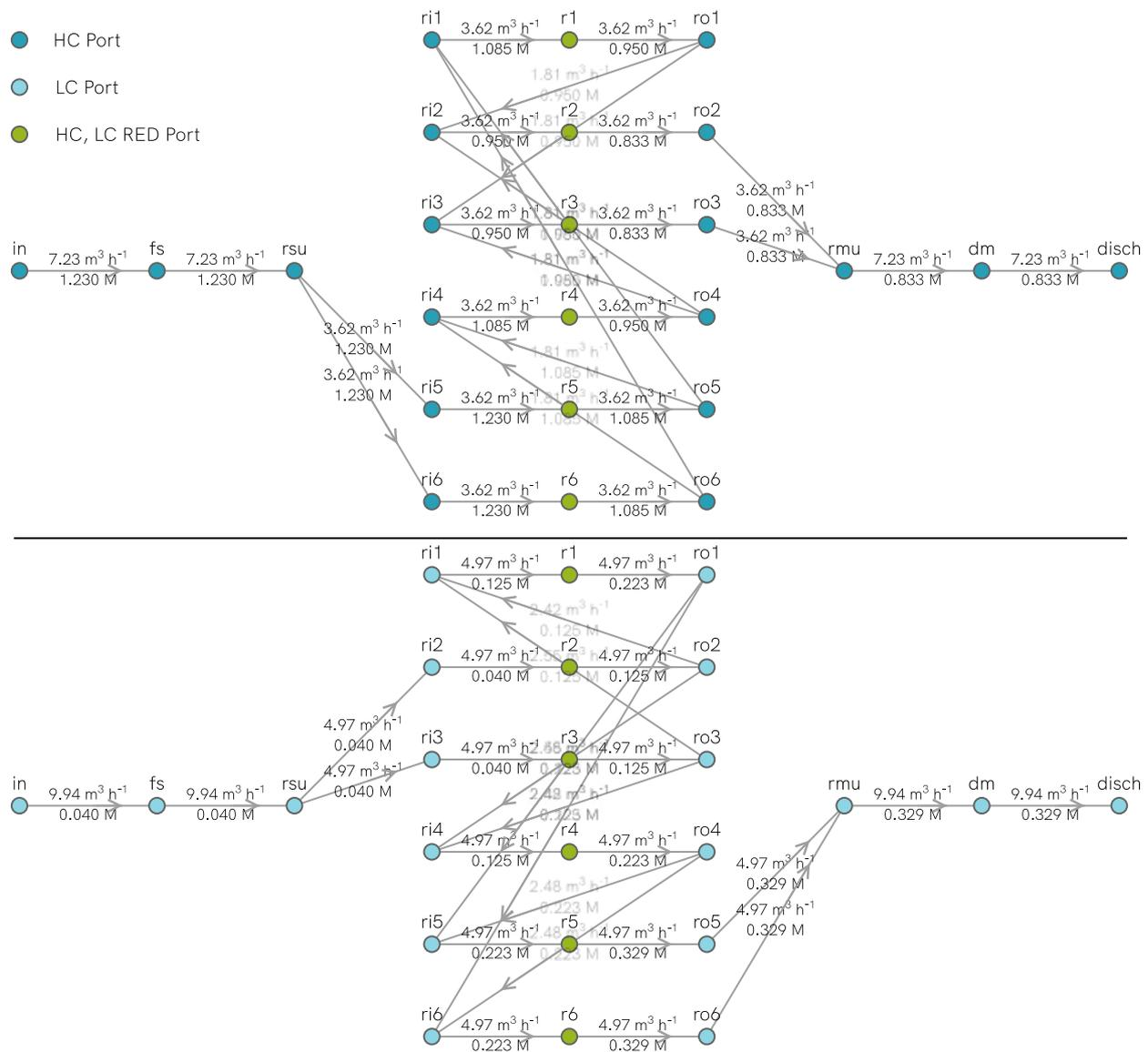
Figure 2 Port connection of a parallel branch in the RED process' optimal flowsheet design. Case study:  $N_r = 15$ ; RED stack working conditions (HC/LC): 1.23/0.04 M, 7.24/9.87  $\text{m}^3/\text{h}$ , 19 °C. GDP (decision) layout; IEMs price = \$1.12/ $\text{m}^2$ .
