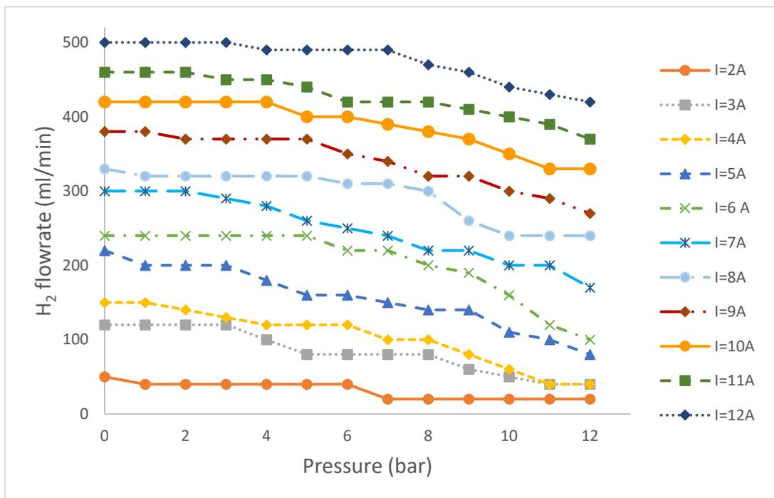
**Figure 12** Hydrogen production as a function of the pressure for different intensities.
