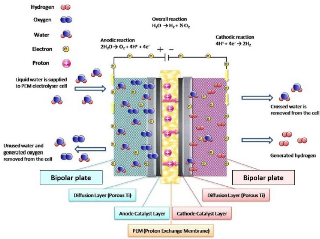
**Figure 5** Working principles and schematic of a PEM electrolyzer.
