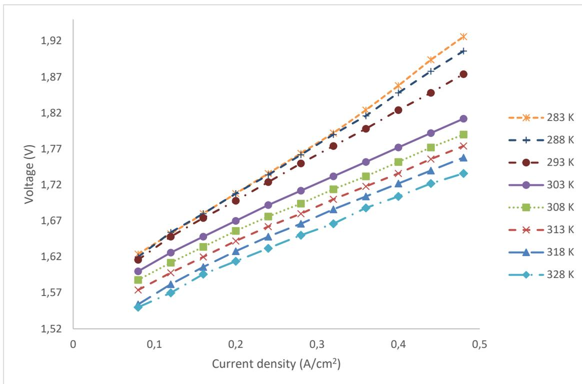
**Figure 9** Polarisation curve at different temperatures.
