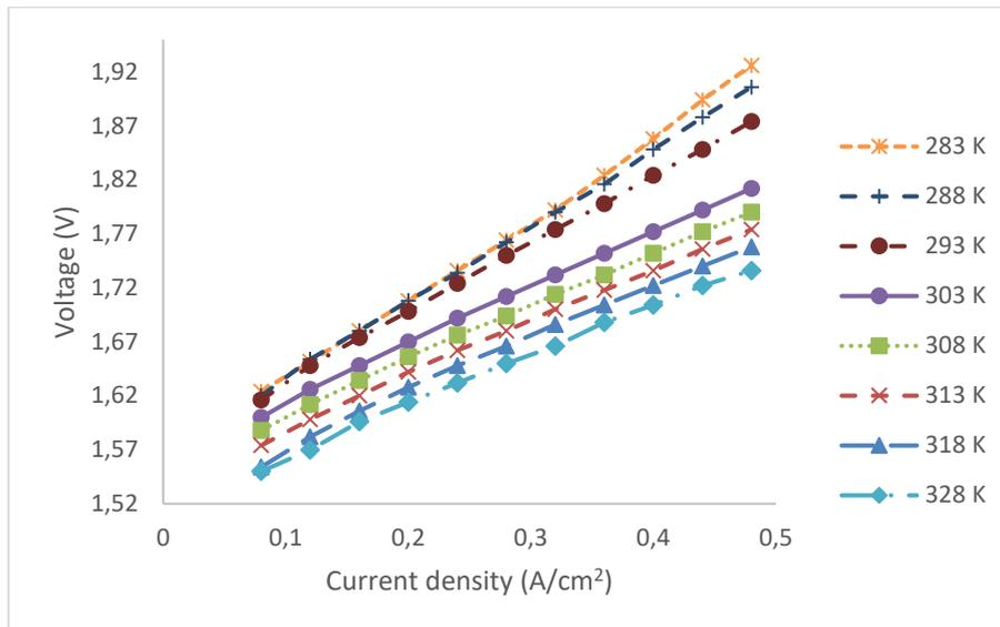
**Figure 1** Polarisation curve at different temperatures.
