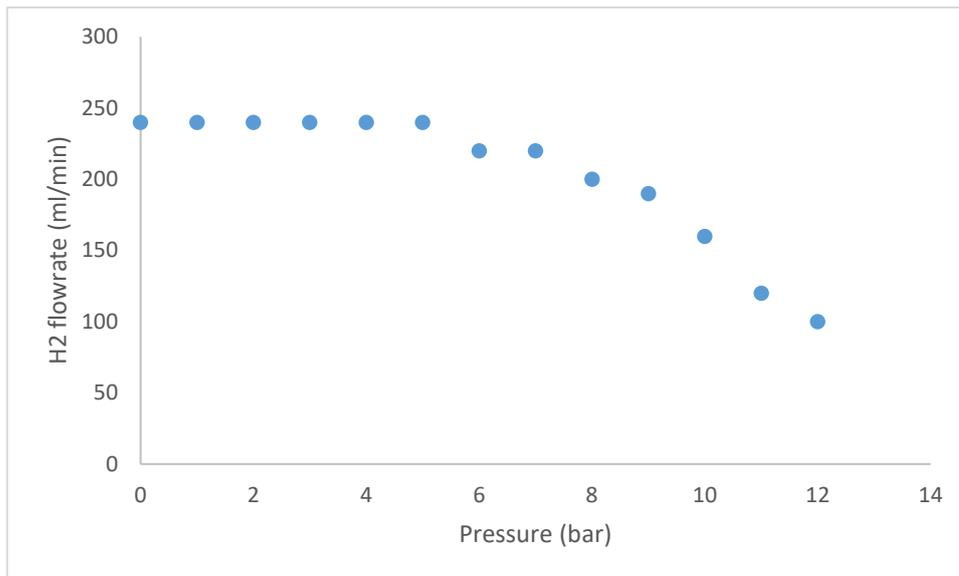
**Figure 11** Hydrogen production as a function of pressure.
