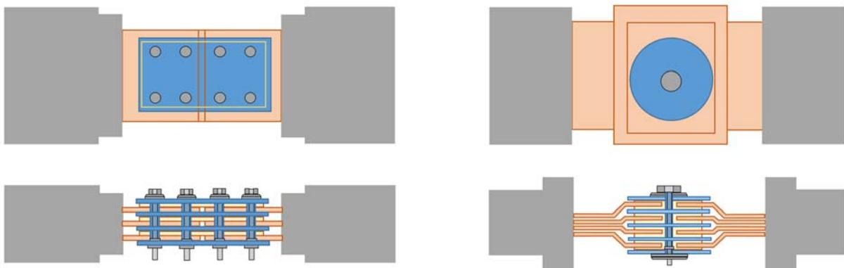
**Figure 4.a.** Traditional (with plates and screws)
