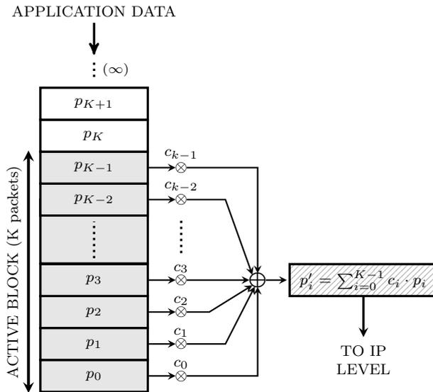
Fig. 1: Coding process (transmitter's RLC layer)
