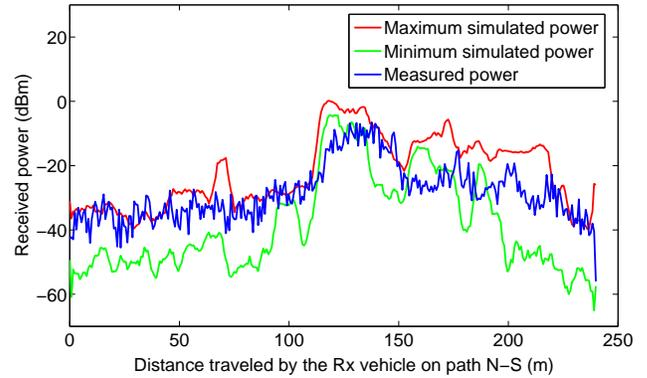
Fig. 2. Simulated and measured power levels when the Rx is moving on N-S path and the Tx is located in position 2.
