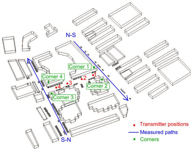
Fig. 1. Layout of the urban environment used in the simulations. The measured paths are depicted by blue, the four Tx positions are depicted by red dots and the corners involved in the simulations are numbered by green.
