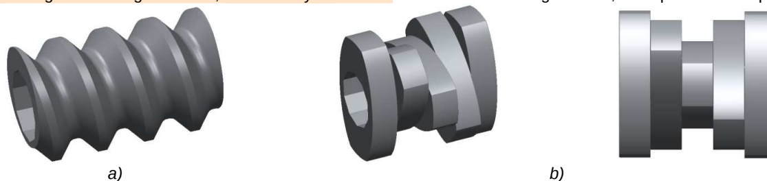
Fig. 3 – Example of screw elements: a) transport element;
