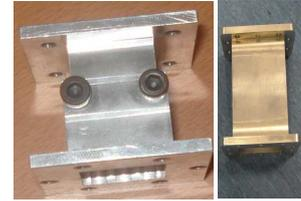
Fig.7. View of the assembled prototypes of both types of the differential phase shifter
