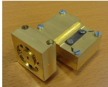
Fig. 7. Total assembly of the complete antenna array
