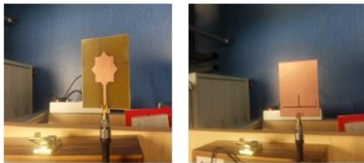
Fig.11. Photo of the fabricated antenna structure
