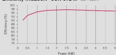
Efficiency INGECON® SUN 5TL M V dc = 680 V
