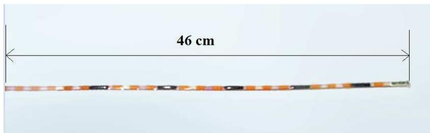
Figure 9: This figure shows a MOSFET linear array, in which the five MOSFET detectors are separated by a orange and white plastic [20].
