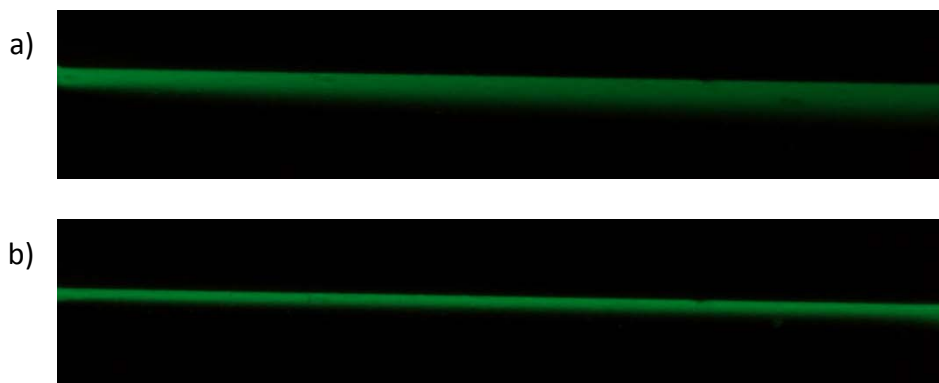
Figure 23. Comparison of phases interface for (a) EXP 1 ( n=4 ), (b) EXP 9 ( n=0.1 ).
