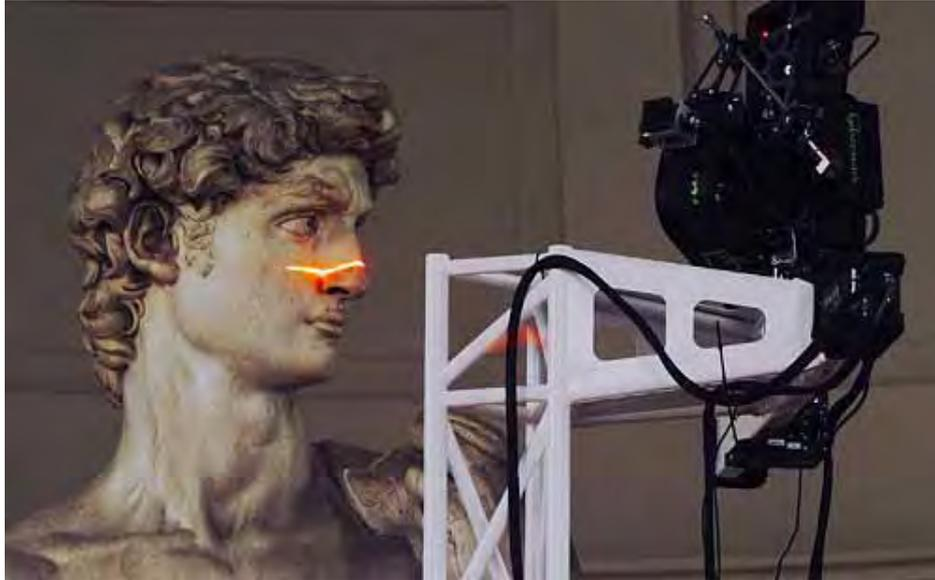
Figure 3.11: The laser scanner used in the *Digital Michelangelo* project to create a digital reconstruction of the famous statue of David (source: *Marc Levoy/Digital Michelangelo Project*).
