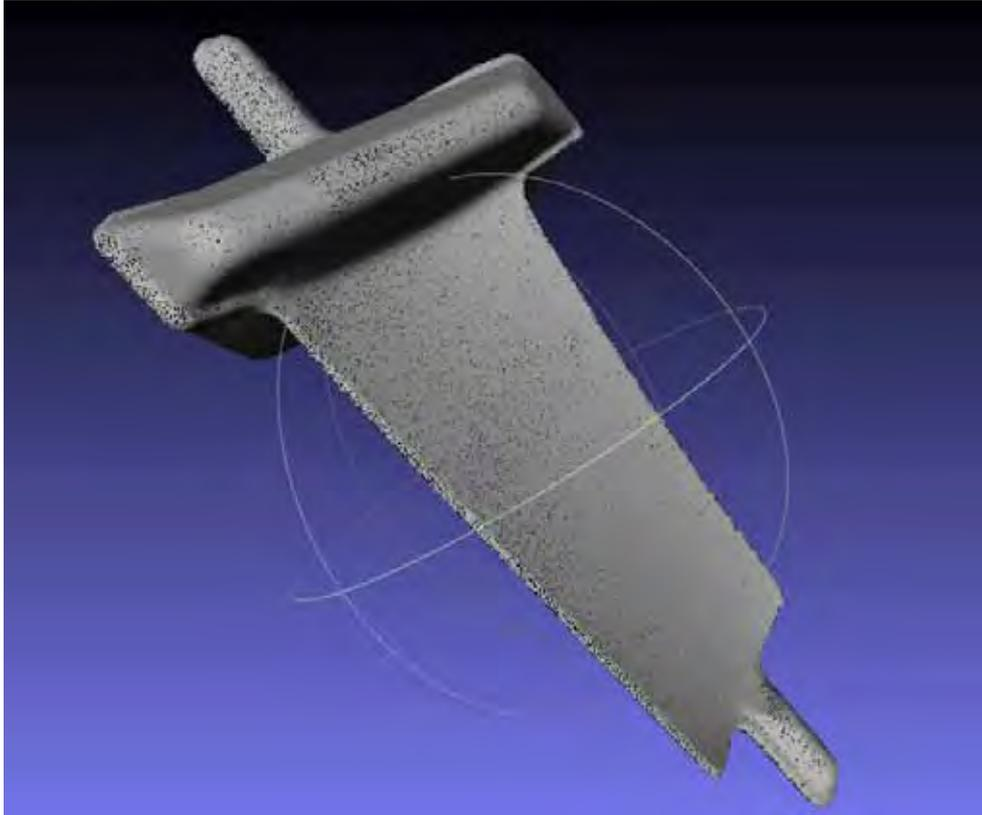
Figure 3.3: Example of a point cloud corresponding to a blade. The model consists of more than 1 million data points.
