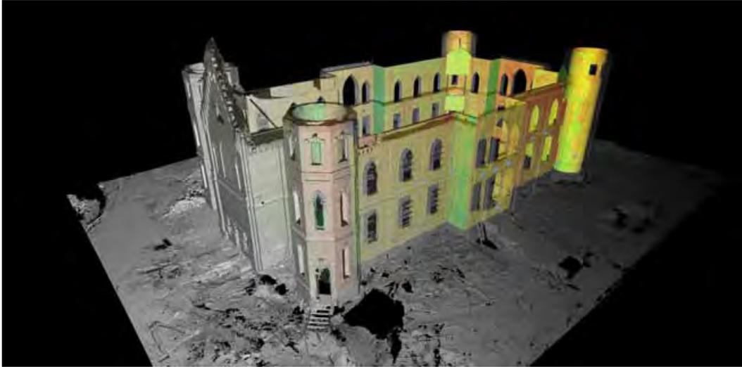
Figure 3.14: Laser scanning used to determine if the facade of this building (destroyed by fire) can still be saved in rebuilding the structure (source: *Diamond Land Surveying*)
