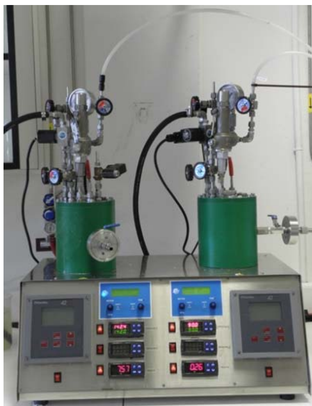
Fig. 2.5 Laboratory digesters used to make the cooking trials.
