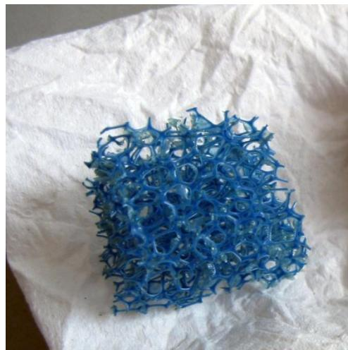
**Figure 3-7** Piece of the sponge type biofilm support
