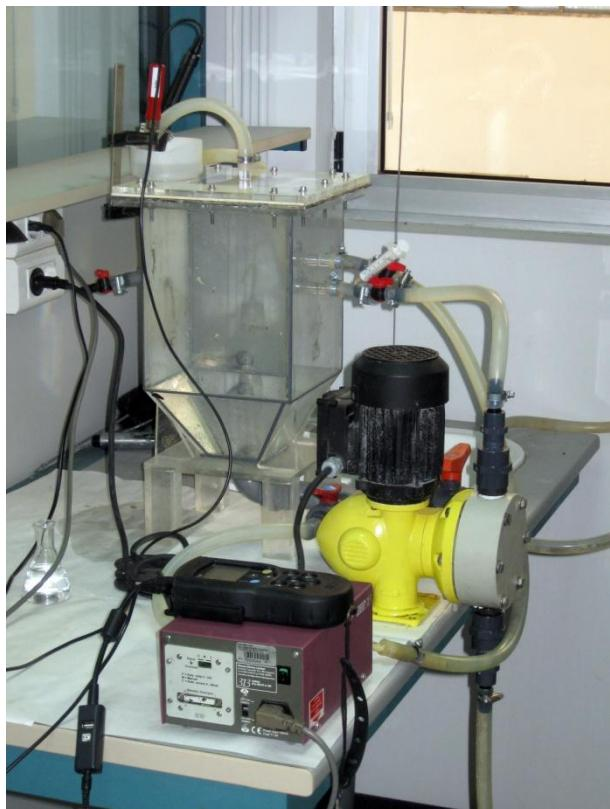
**Figure 3-9** RTD experimental setup for the individual anaerobic zone
