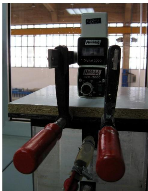
**Figure 3-2** Heidolph RZR-2000 impeller for mechanical mixing in the anoxic zone
