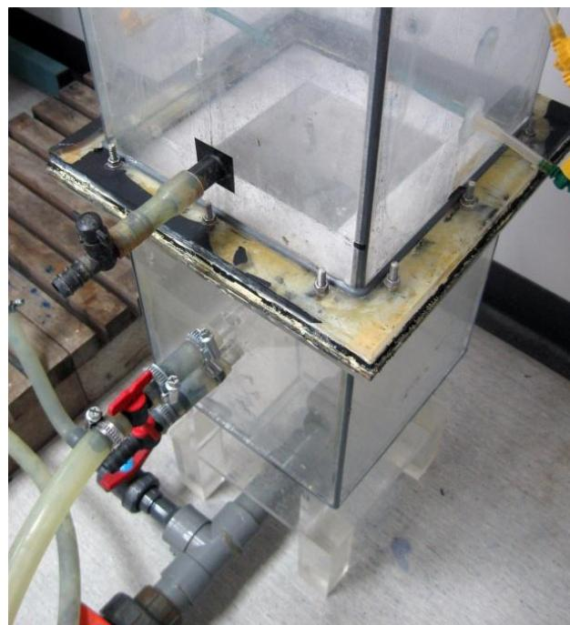
**Figure 3-3** Expanded PVC baffle between the anoxic and anaerobic zones
