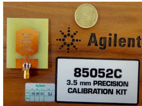
Figure 9- Photograph of the achieved broadband antenna
