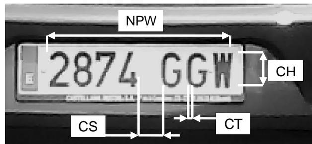
Fig. 3. Number plate parameters. NPW = Number plate width, CH = Character height, CT = Character thickness trace, CS = Characters separation.
