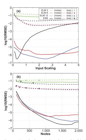
**Figure 4.** Normalized error (in logarithmic scale) of the Mackey-Glass time-series prediction for: (top) ELM and ESN machines with D=1500 neurons and different input scaling values, from 0.1 to 5; (bottom) ELM and ESN models with input scalings 1 and 0.3, respectively. Results for noisy output are indicated by dashed lines.
