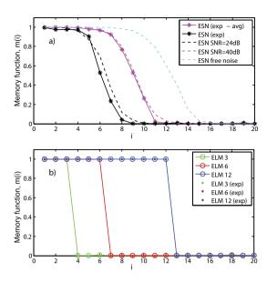
Figure 3. Memory function for the numerical (dashed lines) and experimental (solid lines) realizations of (a) ESN with d=1 and (b) ELM with d=3, 6 and 12, respectively.
