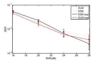
Figure 5. Symbol error rate (SER) for the channel equalization task as a function of the signal to noise ratio (SNR) in the channel. Results obtained with ESN (d=1) and ELM (d=7) for an experimental realization with 40 dB (solid lines) and the corresponding numerical simulations with noise (dotted lines). Discontinuous and continuous lines are mean values and error bars represent two times the standard deviation over 100 realizations.
