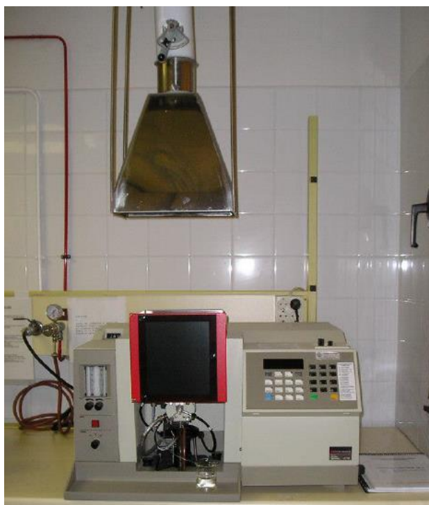
Figure 3.3. FAAS equipment: Perkin Elmer 3110B
