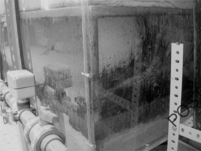
Figure 5. Oil adhesion to the SCPT inner walls.
