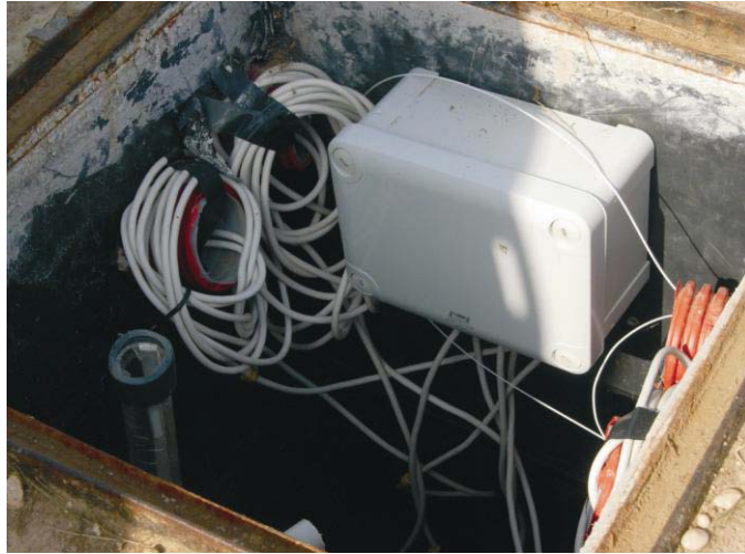
Figure 4. Register box with datalogger and temperature probes
