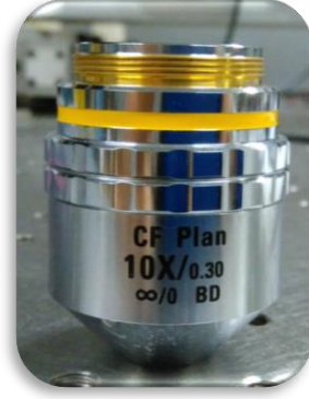
Figure 3.3: microscope objective with a 10x magnification.
