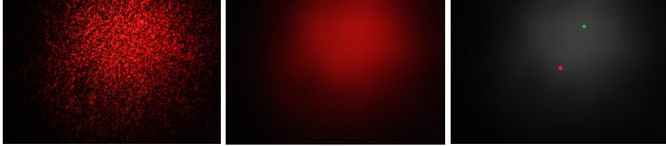
Figure 5.3: from left to right, original image taken with the camera, image after applying a low pass filter ( r = 100 \text{ pix.} ) and image in grey scale: Red points shows the coordinates' origin and green point shows the maximum of the distribution.
