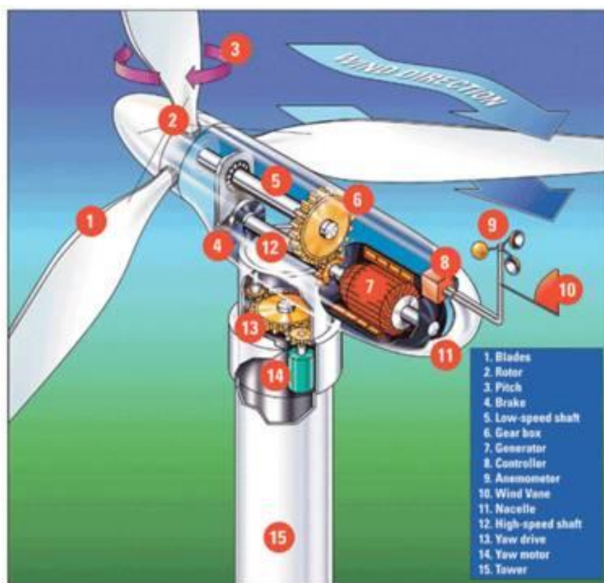
3.21. Scheme of a powerful wind turbine. Source: http://www.reuk.co.uk/
