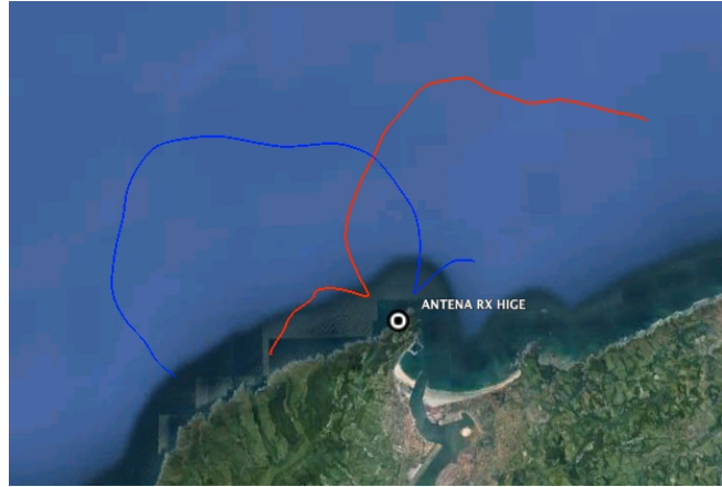
Figure 23: Measured HF radar antenna patterns of Matxitxako (2014) and Higer (2011) Sites over Google Earth maps.
