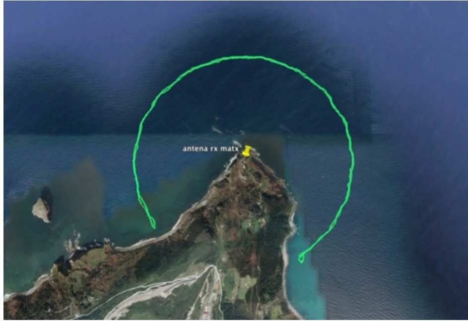
Figure 14: Trajectory (in green) of the boat with the transponder on board to calibrate the antenna of Matxitxako in September 2014. Yellow marker shows the position of the receiving antenna (courtesy of Qualitas Remos).
