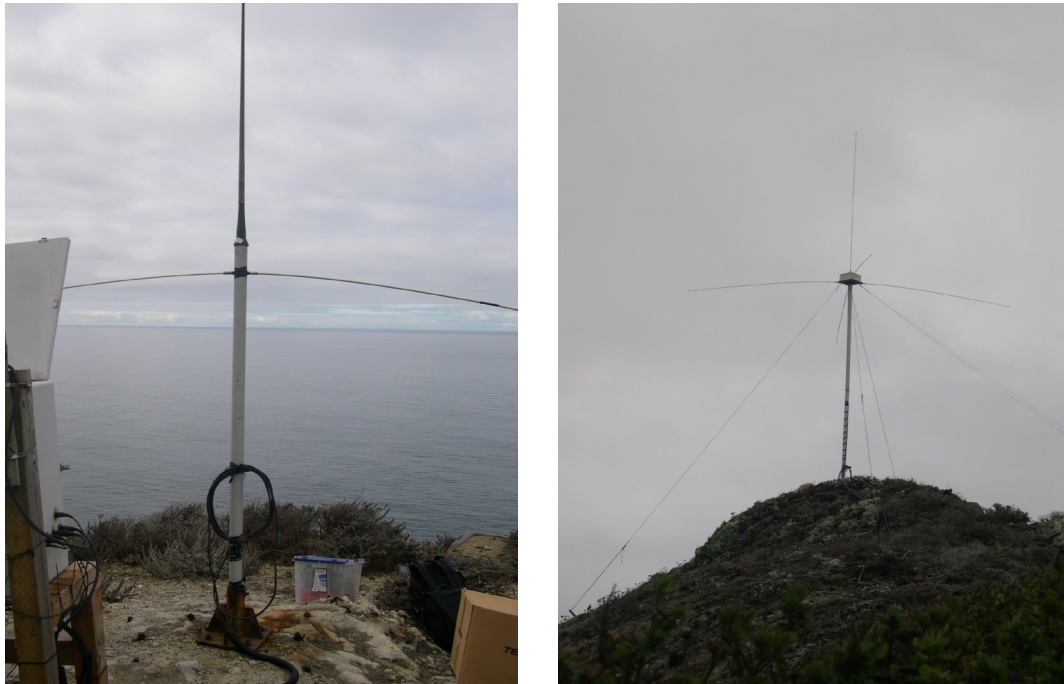
Figure 10: HF radar antennas (CODAR system) at Point Sur in California; transmitter (left) and receiver (right)
