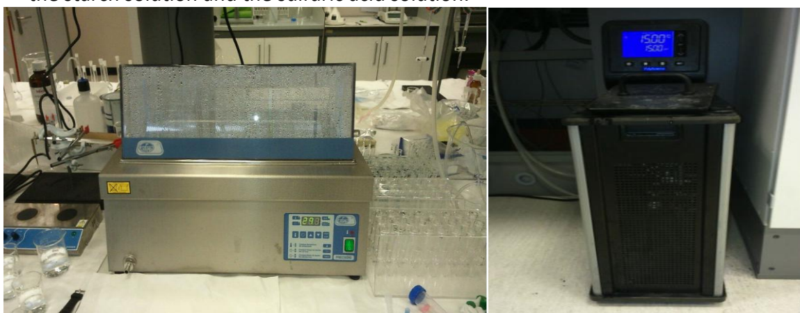
Figure 11. Thermostatic bath (20 °C, 22.5 °C, 25 °C, 28 °C and 30 °C) (on the left) and cooling bath with thermostat (15 °C) (on the right).
