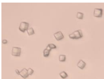
Figure 4.10. Continuous crystallization, [IL] = 100 mg/ml, T=20°C, cubic geometrical crystals, No agglomeration
