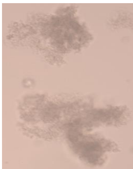
Figure 4.9. Just Precipitation. Experiment without Ionic Liquid at 7°C
