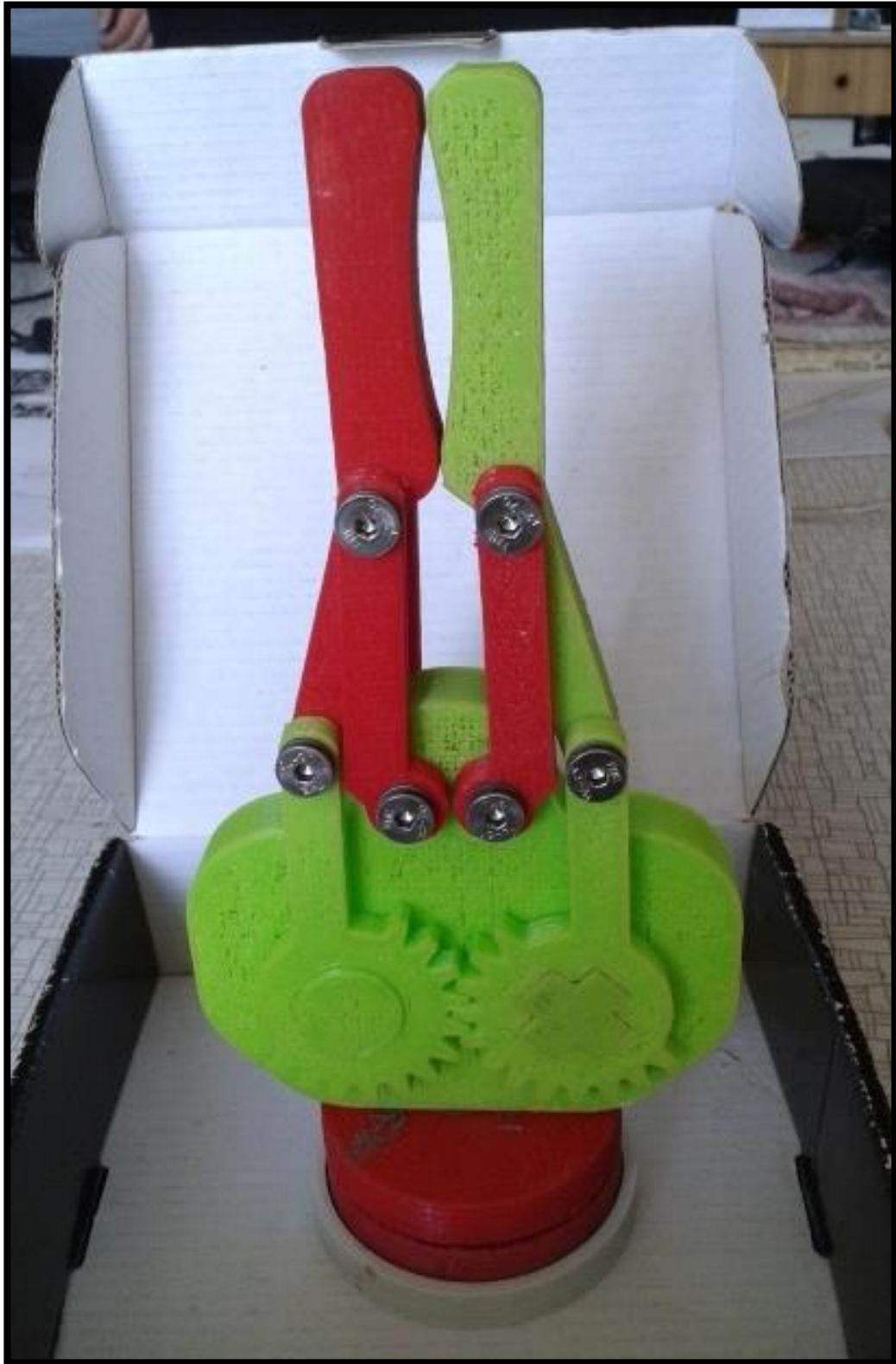
[74] – Picture of the real gripper with the minimum aperture
