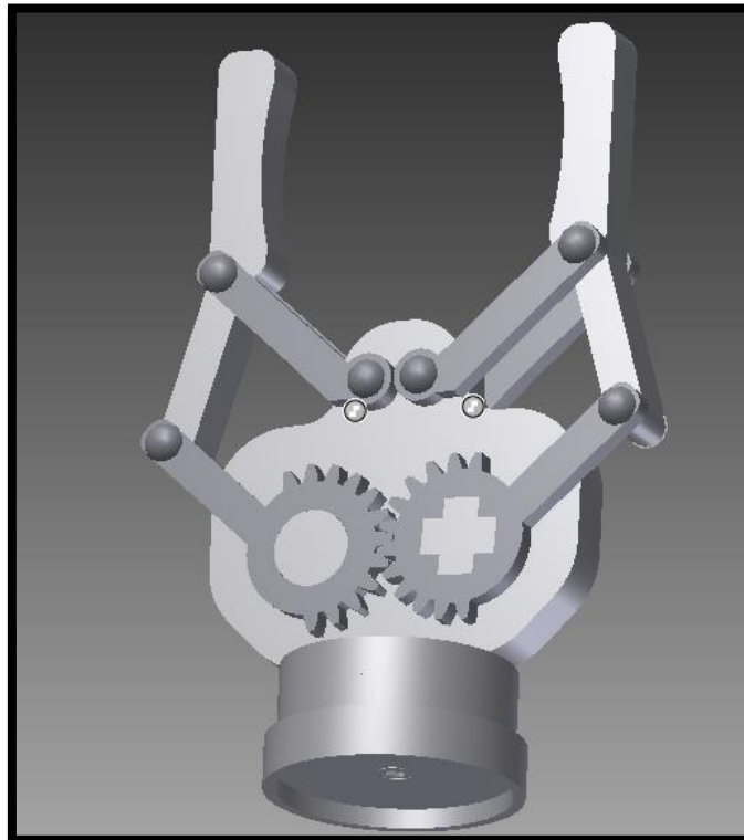
[24] – Perspective view of the last design of the gripper
