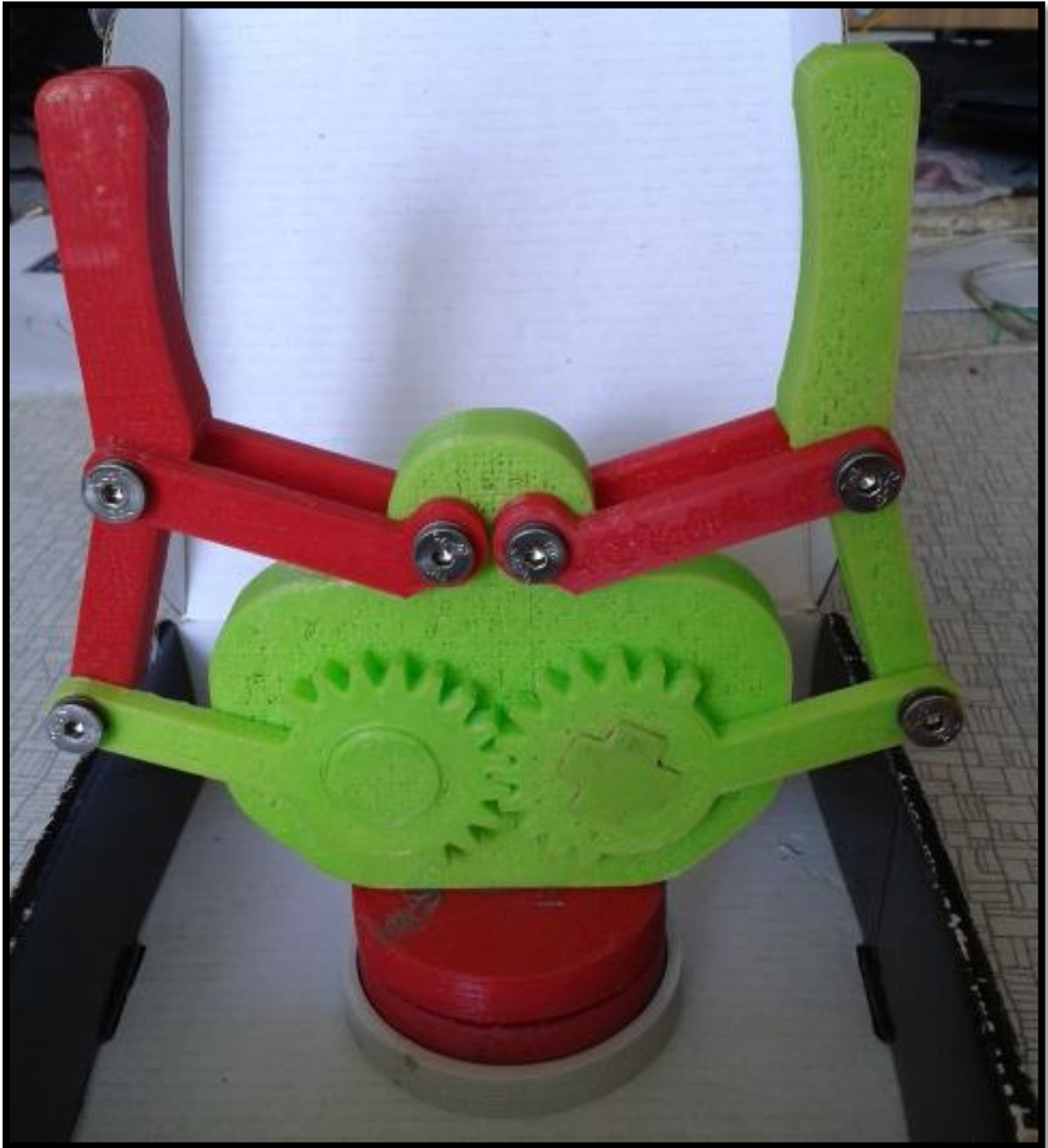
[75] – Picture of the real gripper with the maximum aperture
