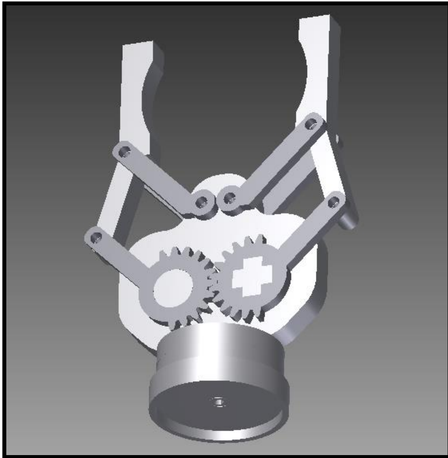
[22] – Perspective view of the third design of the gripper
