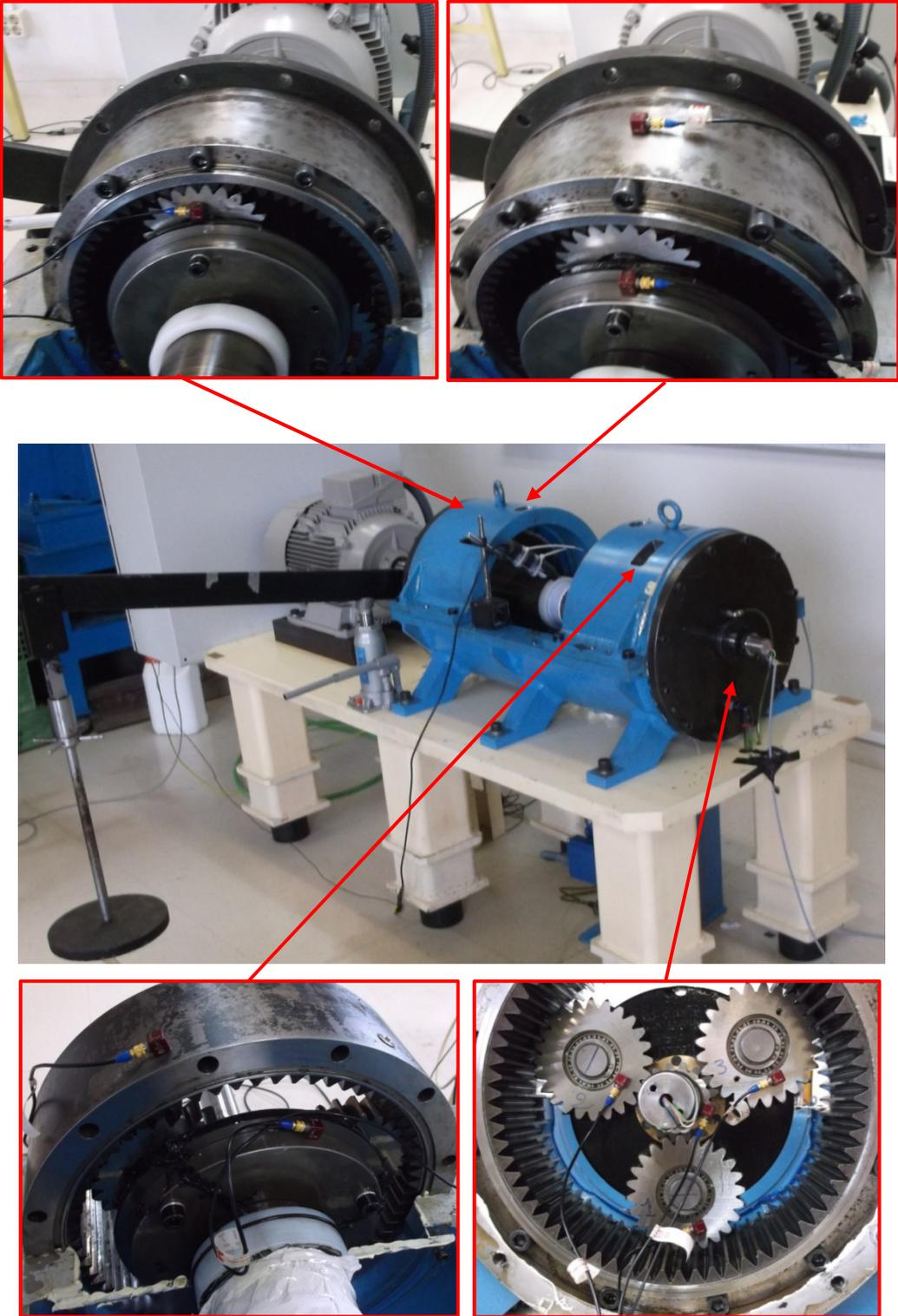
**Fig 5.14:** Accelerometers mounted in components of the back-to-back planetary gear
