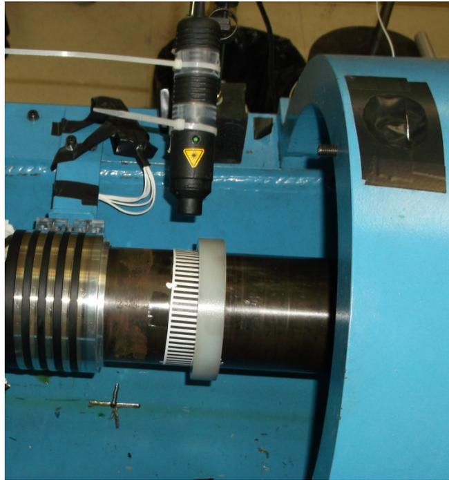
**Fig.2.11:** Optic tachometer
