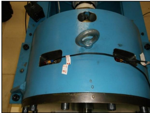
**Fig.2.9:** Tri axial accelerometers on the test ring
