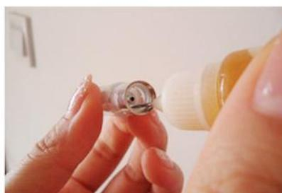
2 Target the tube interior wall with the liquid injection bottle
