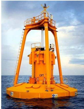
**Figure 2.6:** Ocean Power Technology Power buoy, see Ocean Power Technologies Web page
