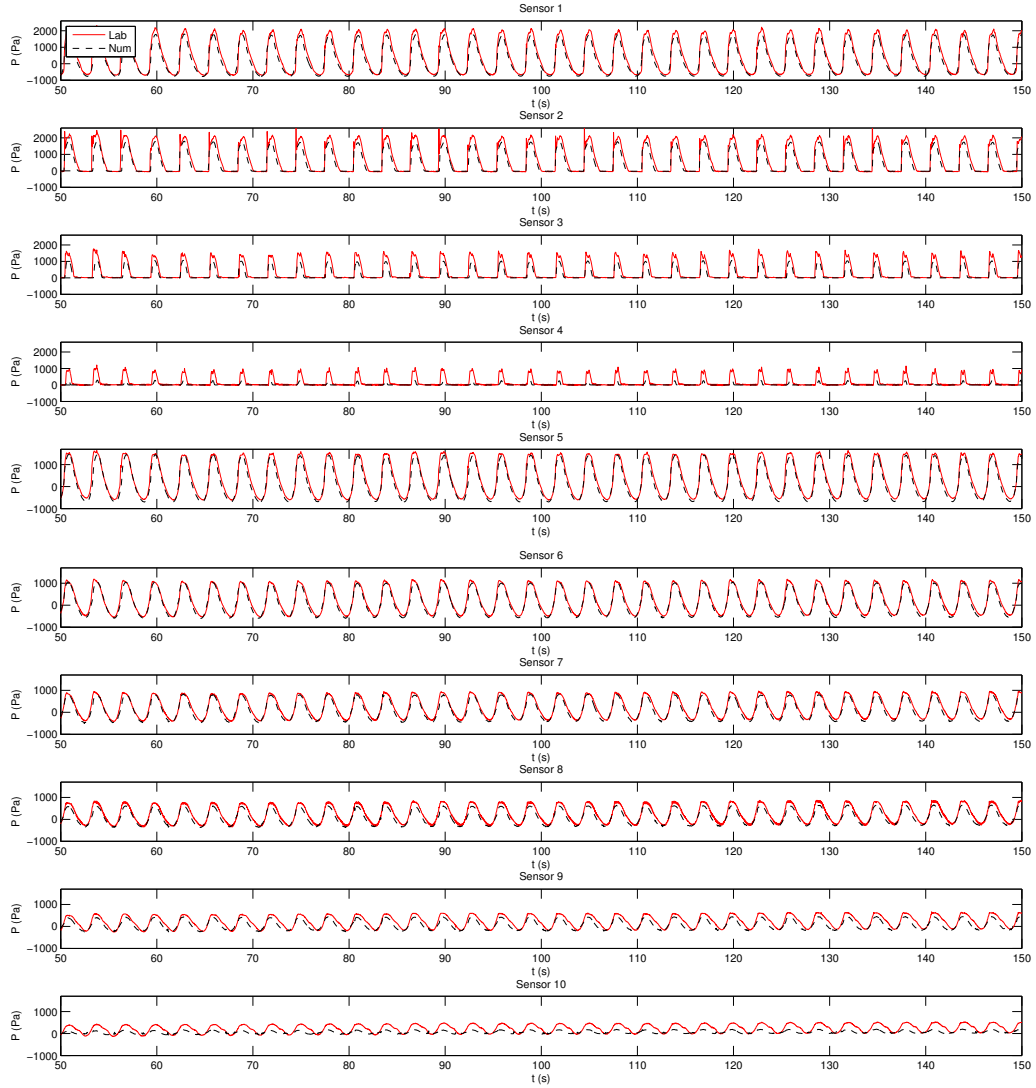
Figure B.4: Regular waves interacting with a high mound breakwater in 2D: pressure series. del Jesus et al. (2012) formulation.
