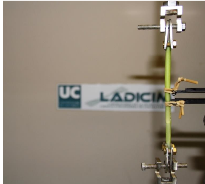
Figure 4.5 Tensile strength test for S. anglica stem.
