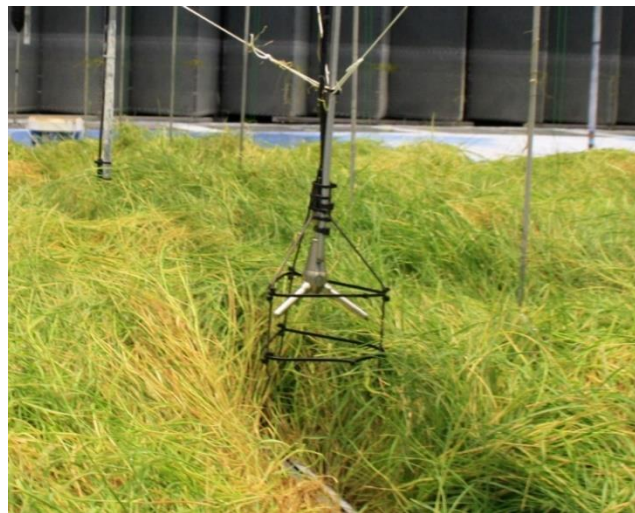
Figure 4.8 Special structure built around the ADV
