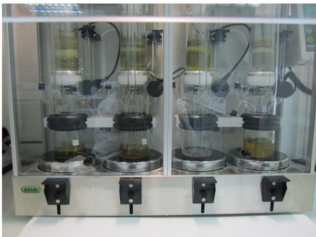
Figure 3.9: B-811 Büchi Extraction unit during extraction process.
