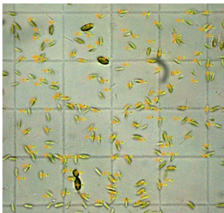
Figure 3.5: Thoma chamber grid during the cell direct counting under optical microscope.
