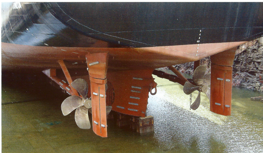
Fixed-pitch main propellers, Becker rudders and stern tunnel thruster in research vessel James Cook
