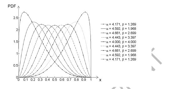
Figure 3. Beta-PERT PDFs for the 3-tuple  $[x_{min}, x_{m.l.}, x_{max}]$  on the interval [0, 1]
