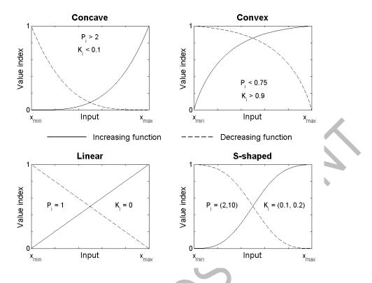
Figure 1. Different shapes and parameters of the MIVES method
