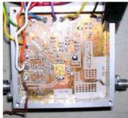
Figure 5.79: Photo of the test board assembled inside the metallic box.
