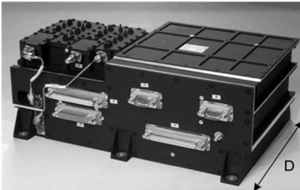
Figure 5.99: Old generation of S-Band TT&C transponders
