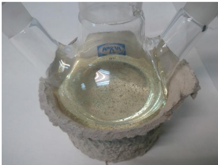
Figure 2.2: 10% w/w PAN solution in NMP filtered and ready for degassing
