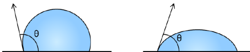
Figure 2.4: Measurement of the contact angle
