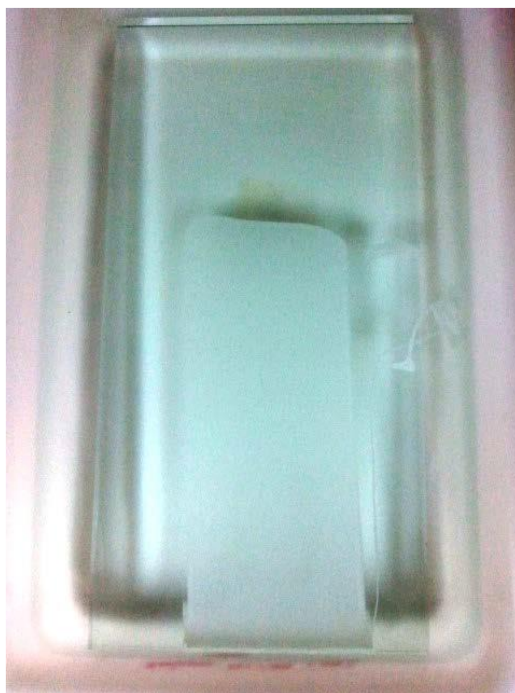
Figure 2.3: Glass plate and PAN polymer solution immersed in the coagulation bath for the exchange of the solvent and non-solvent to promote the PAN precipitation
