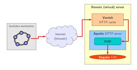
**Fig. 1** GeoGebra communicates with SingularWS via the HTTP protocol. Caching layer software Varnish can also be inserted to speed up classroom usage when the same queries may be sent by more students, but only one computation is preferred for all of them. Newest version of SingularWS itself can maintain caching without any extra software required.
