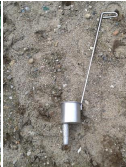
Figure 32-Extraction tool used in the ISM
