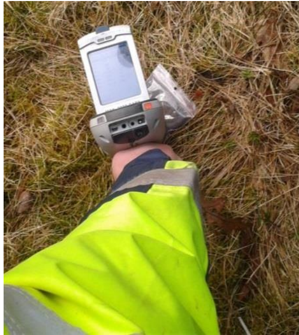
Figure 28- Handheld XRF used in the testing
