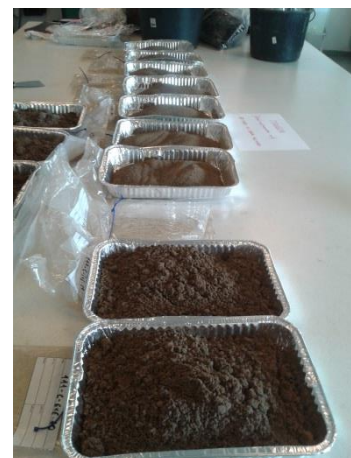
Figure 65- Samples after granulometry division
