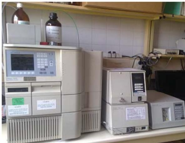
**Figure 2.1. High-performance liquid chromatography system Waters 2690 Separation Module.**
