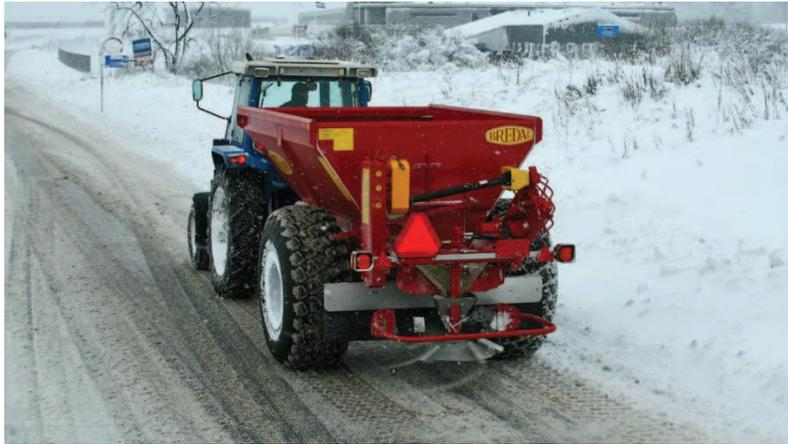
Figure 1. Spreading salt on icy road (BREDAL A/S 2014)
