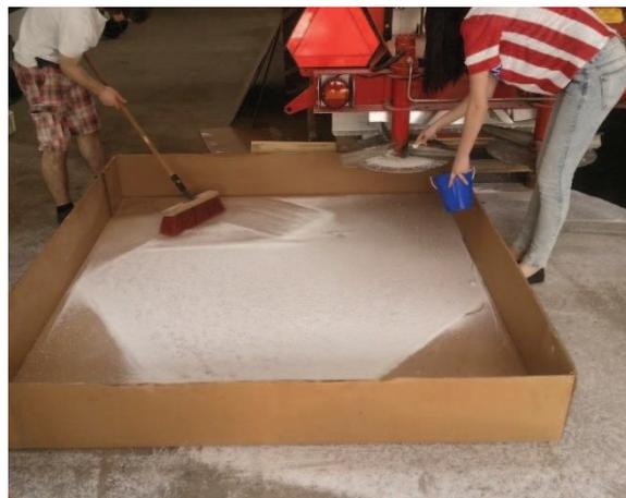
Figure 36. Measurement of mass flow in progress
