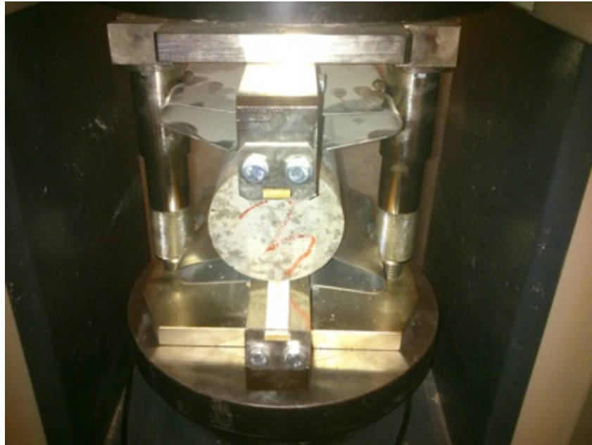
Figure 31. Placement of the cylinder for the splitting tensile strength test
