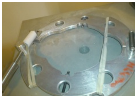
Figure 33. Circumferential extensometer for measuring transversal strain
