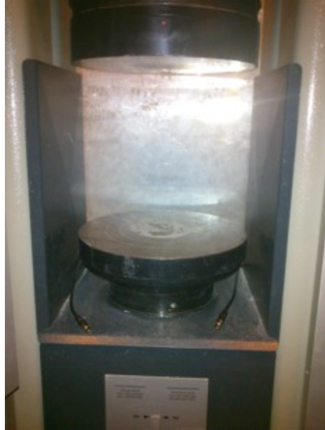
Figure 29. Machine ready for the splitting tensile strength test
