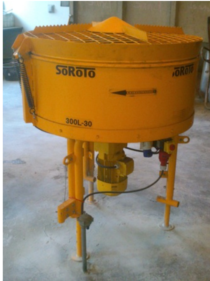
Figure 17. Machine used for mixing concrete
