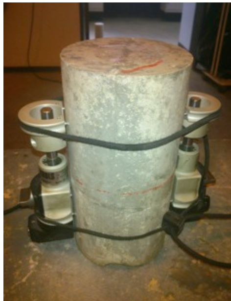
Figure 32. Gauges for measuring longitudinal strains
