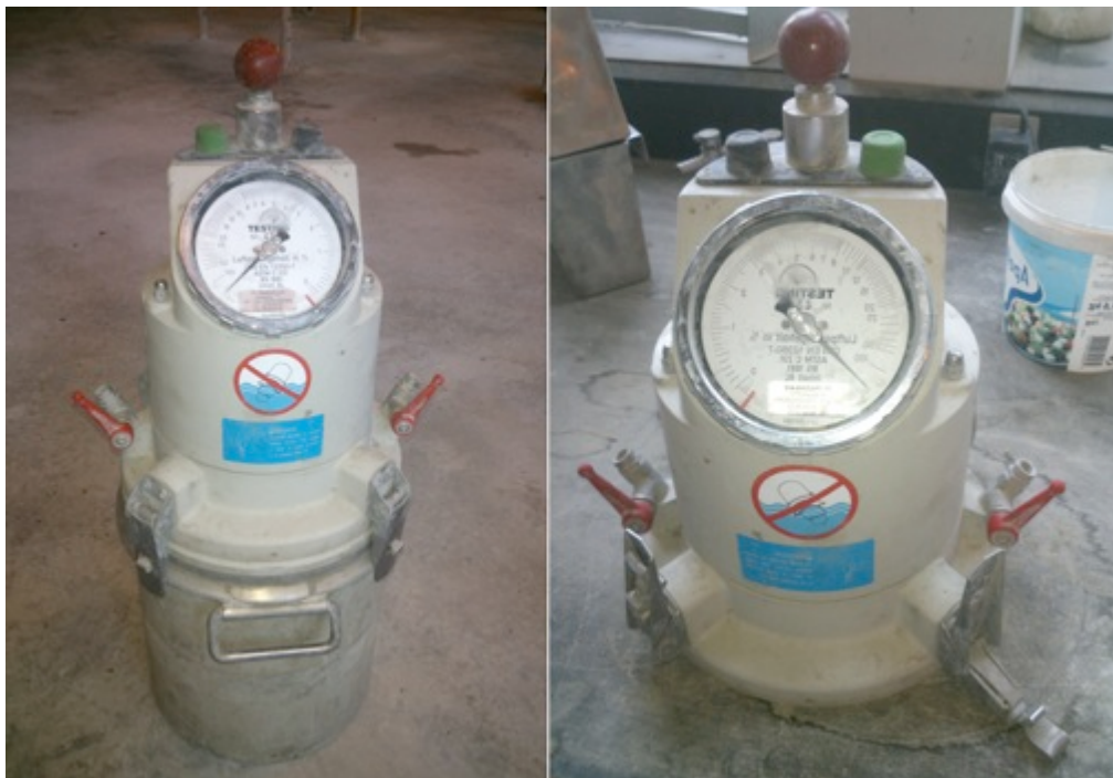
Figure 21. Device to measure the air content in fresh concrete
