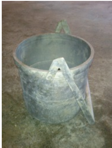
Figure 18. 10 litres bucket for measuring fresh concrete density
