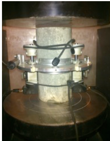
Figure 34. Extensometers for measuring longitudinal and transversal strains
