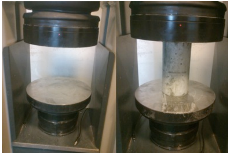
Figure 28. Compressive strength test
