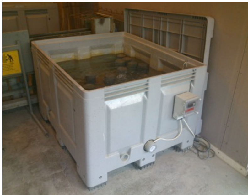
Figure 25. Tank filled with water for concrete curing at 20°C
