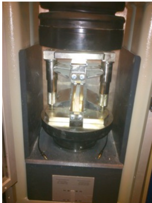
Figure 30. Splitting tensile strength test
