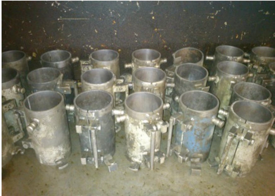
Figure 22. Moulds used to make concrete
