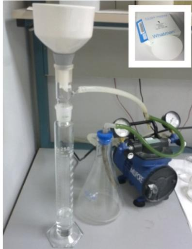
Figure 2-4 A picture of the Buchner funnel test and detail of filter paper
