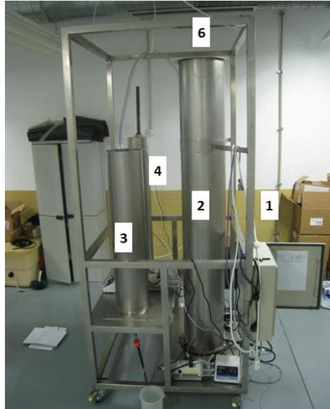
Figure 6-1 (up) Schematic diagram and (down) picture of the combined UASB-HMBR system: (1) Feeding, (2) UASB stage, (3) Anoxic compartment with Kaldnes K3 filter media, (4) Membrane filtration compartment, (5) Permeate (backwashing), (6) Biogas outlet.
