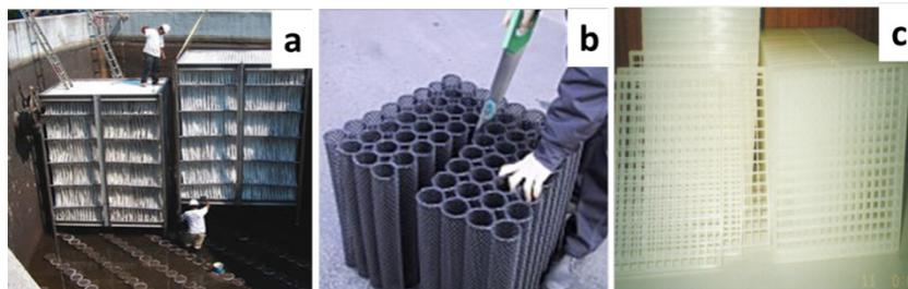
Figure 1-3 Fixed bed support media used in SFBBR: (a) Ropes or nets AccuWeb Brentwood Industries, (a) EXPO-NET's BIO-BLOK® and (c) BLAS®.
