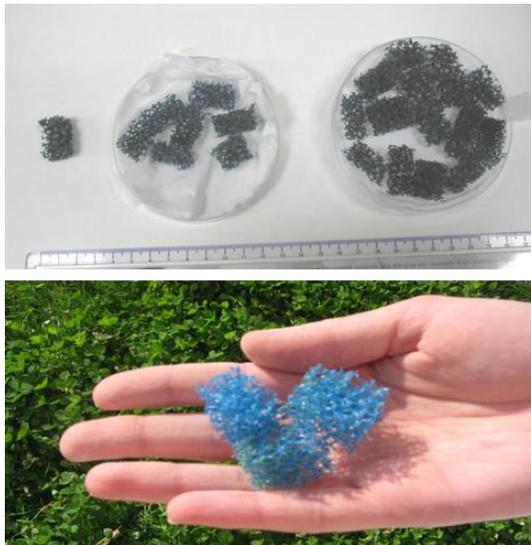
Figure 3-3 Aqua Medic support media without biofilm
