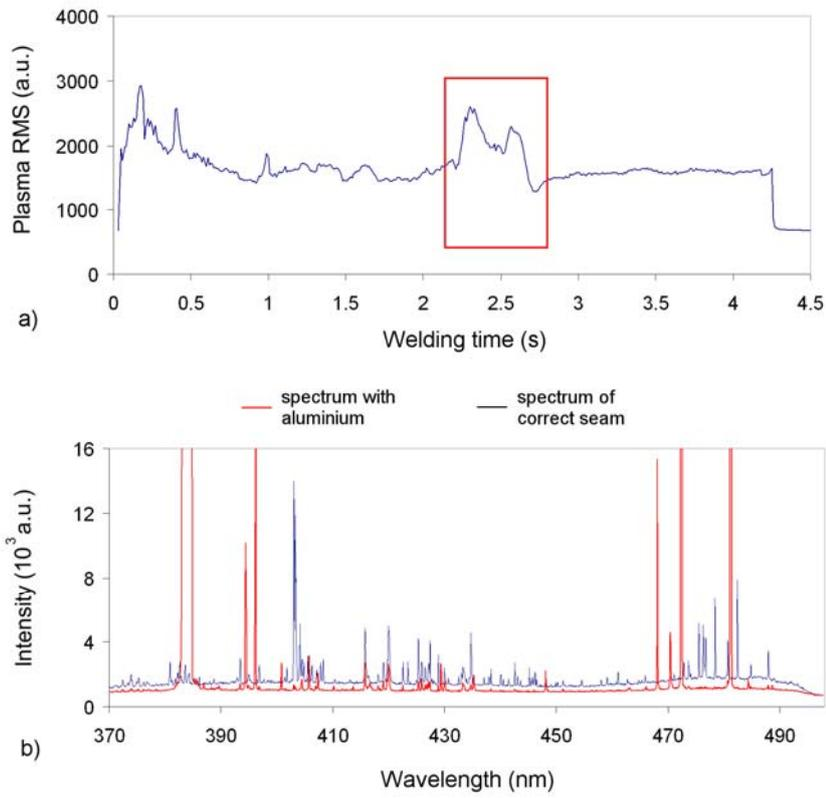
Fig.2: Plasma-RMS profile and spectra of seam with aluminium
