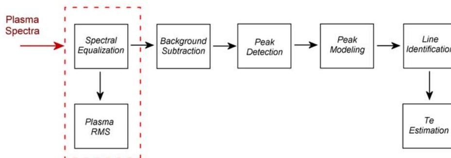
Fig. 1: Processing stages required to obtain  $T_e$  and Plasma-RMS
