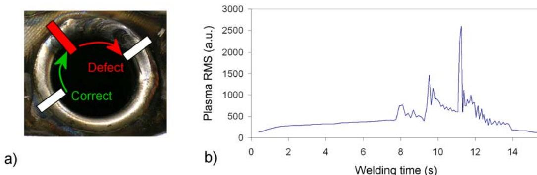
Fig.4: Plasma-RMS for orbital tube-to-tubesheet defective seam
