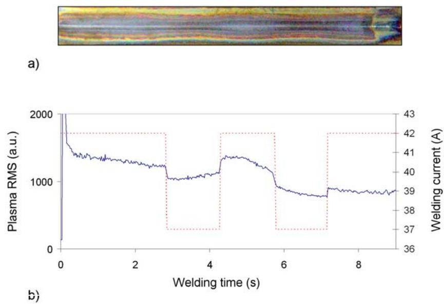
Fig.3: Plasma-RMS profile for seam with different welding currents.
