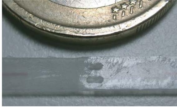
**Fig. 4.31.:** *Manufactured sensor previous to its installation. The left side of the sensor is covered with polyvinyl alcohol to prevent bonding of the section.*
