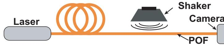
**Fig. 5.18.:** A shaker has been placed close to the multimode fiber.
