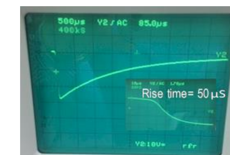
Figure 6. Voltage Waveform and gradient: Rise time \approx 50 \mu s Decay time \approx 5 ms The magnitude and gradient of magnetic field produced by the device can be adjusted through variable resistance and inductance.
