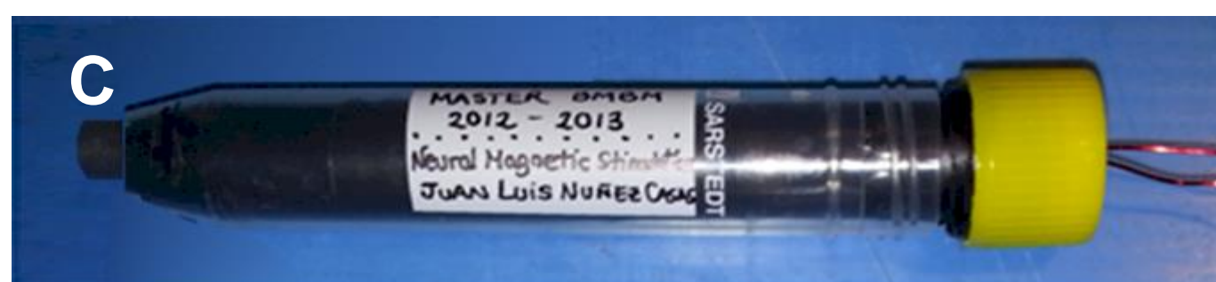
Figure 2. Scale Prototype: (C) Solenoid coil built
