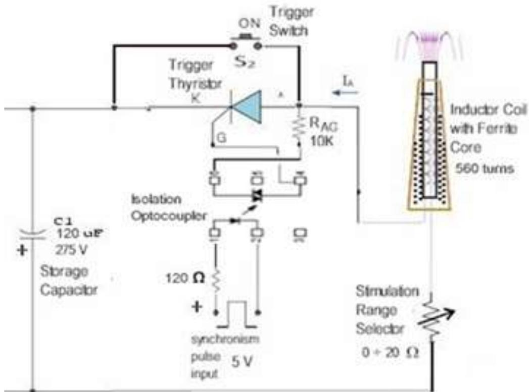
The magnetic discharge system is a classic RLC (resistor-inductance-capacitor) oscillator circuit.
