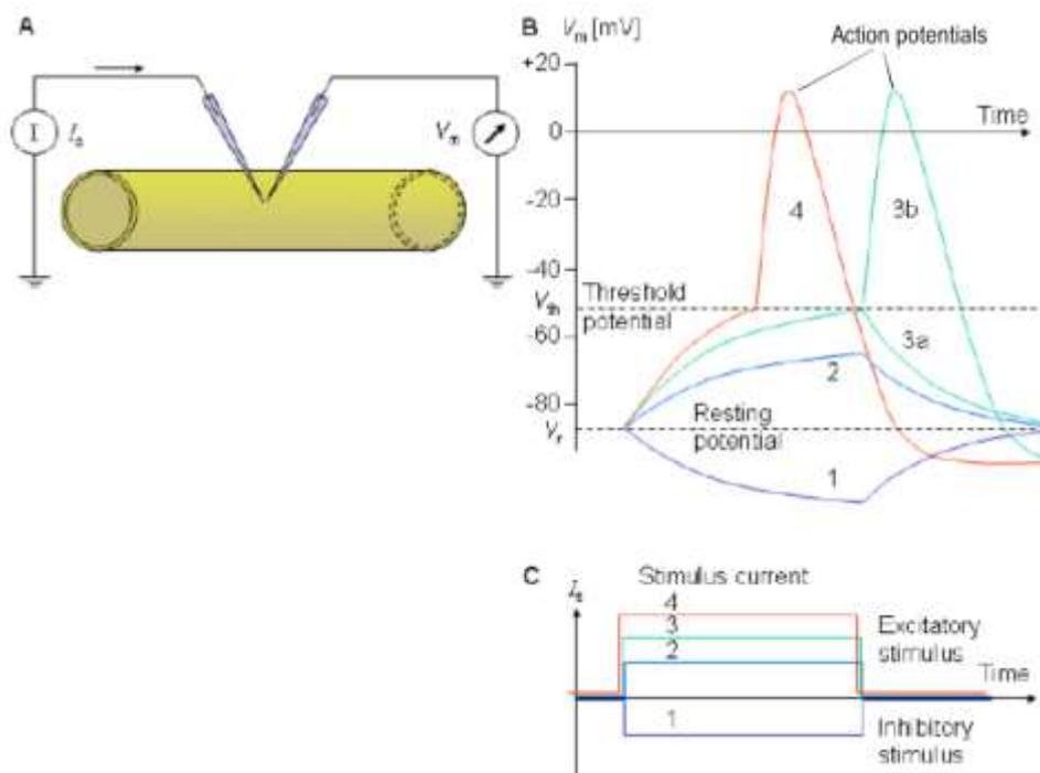
Fig. 4. (A) Experimental arrangement for measuring the response of the membrane potential; (B) Inhibitory (1) and excitatory (2, 3, 4) stimuli. Ref. (4).
