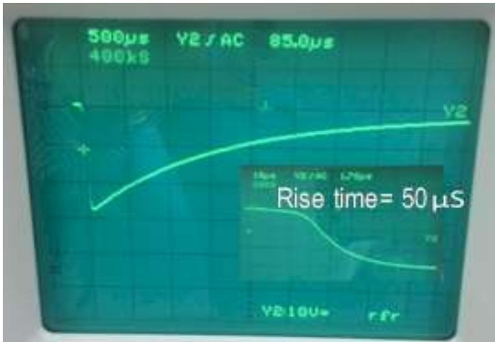
Figure 19. Voltage Waveform and gradient:
