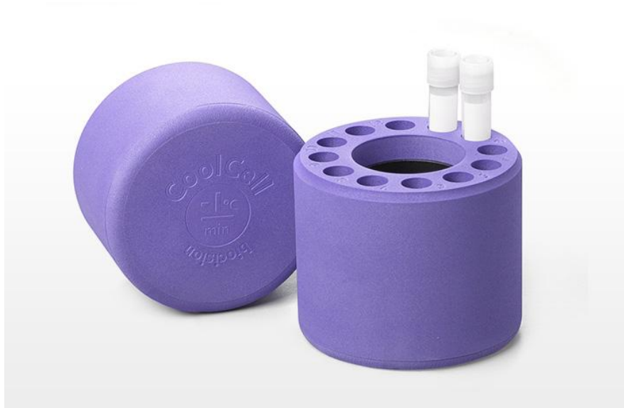
Figure 5: Container to freeze PBMC in cryotubes slowly, named Coolcell®.
