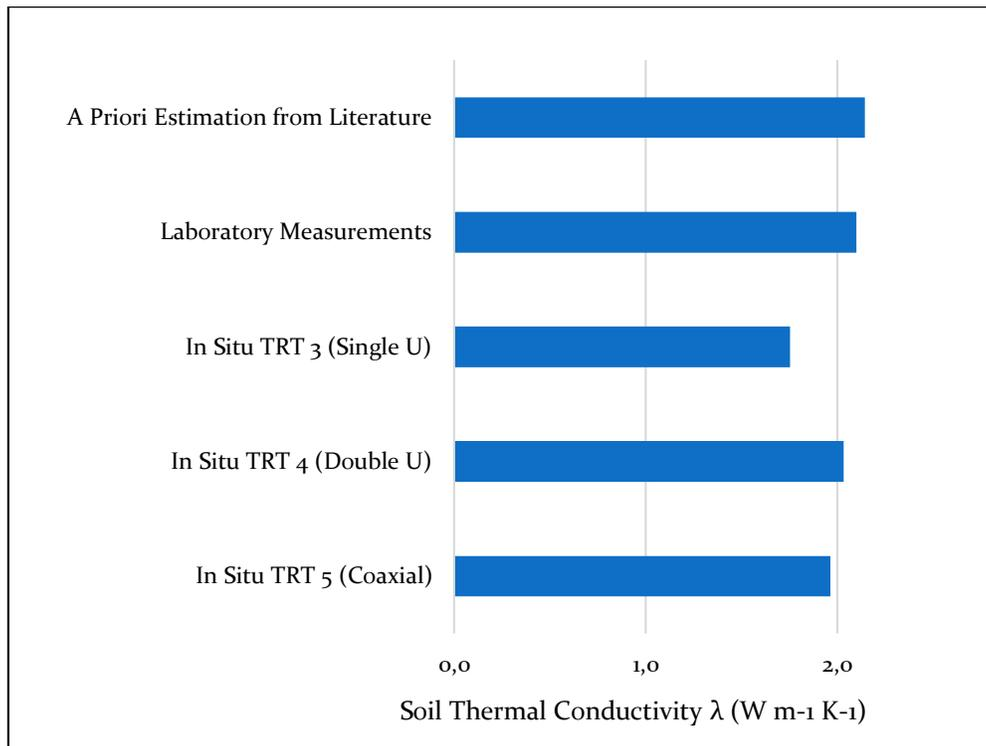
*Figure 5.1-1: Comparison between thermal conductivity values estimated from the literature, laboratory measurements and in situ TRT.*
