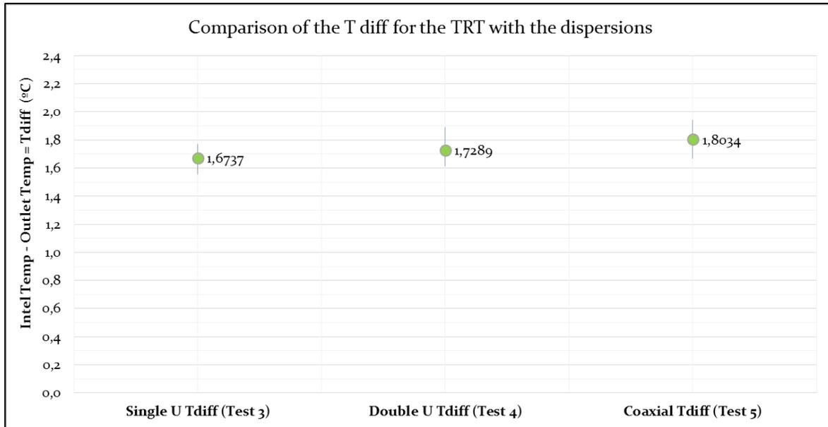
Figure 4.3-16: Comparison of the mean deduction values between the inlet and outlet temperatures together with their dispersions.
