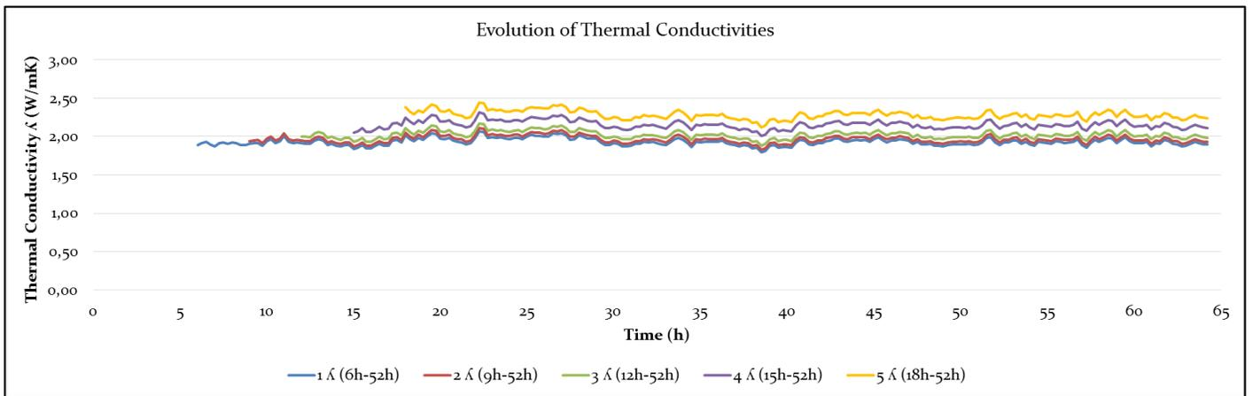
Figure 4.3-11: Evolution along time of thermal conductivities for each period in Test 5.
