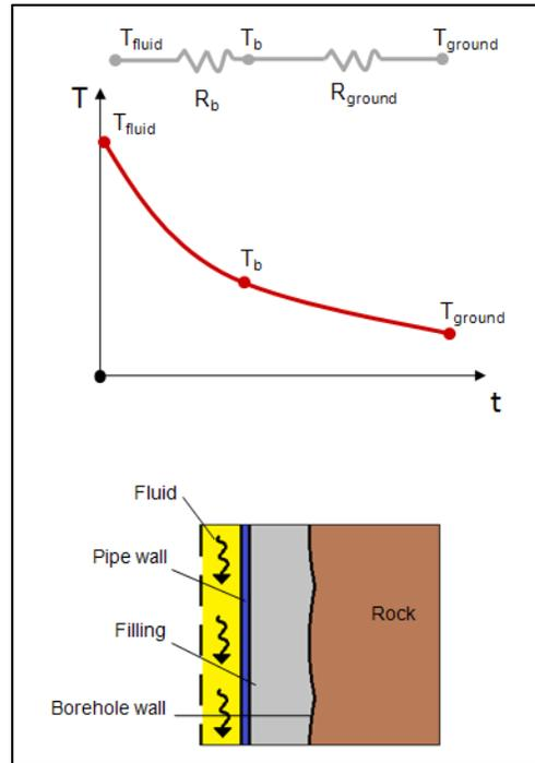
Figure 2.2-2: Thermal resistance fundamental in borehole heat exchanger (Monzó 2011).
