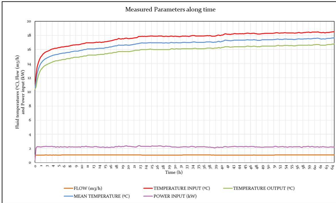
Figure 4.3-9: Measurements along test time for Test 5.
