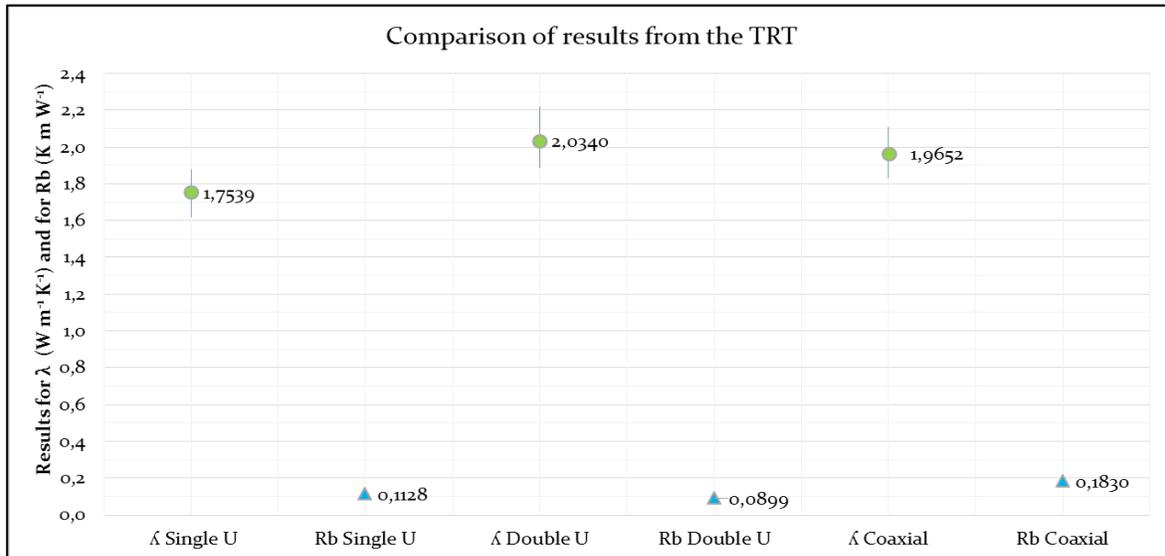
*Figure 4.3-13: Comparison of results for the three TRT.*
