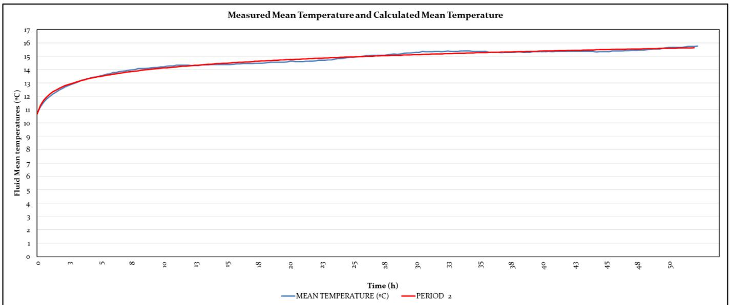
Figure 4.3-8: Fitting curve between measured meand temperature and the calculated one for period 2 in Test 4.
