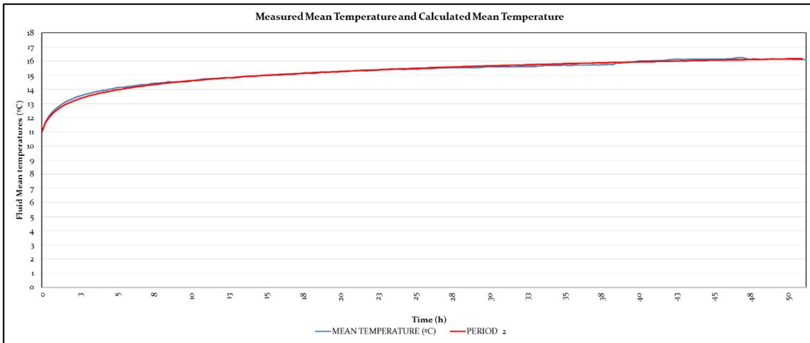
Figure 4.3-5: Fitting curve between measured mean temperature and the calculated one for period 2 in Test 3.
