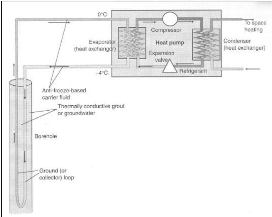
*Figure 2.2-3: A schematic diagram of an indirect circulation closed-loop scheme, installed in a borehole (Banks, 2008).*
