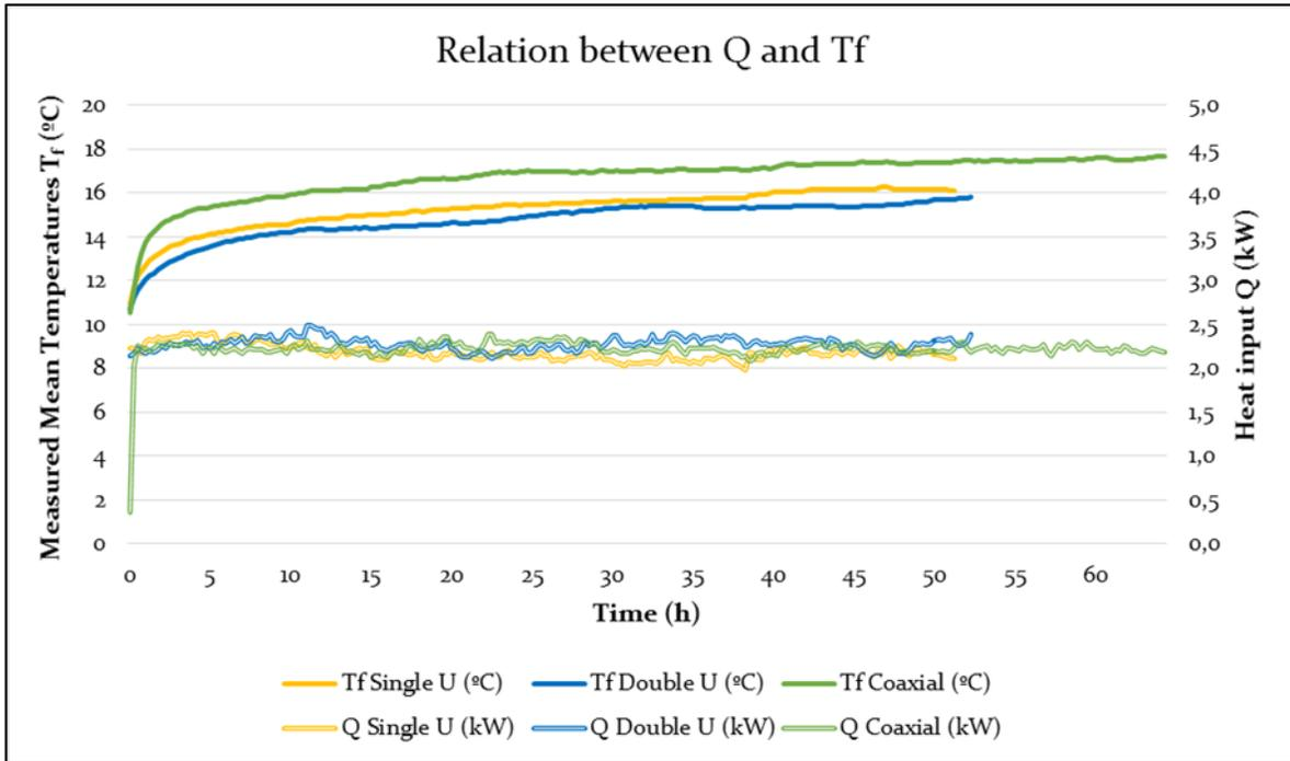
Figure 4.3-14: Graph showing the measured mean temperatures and the heat injection rate for the three tests.
