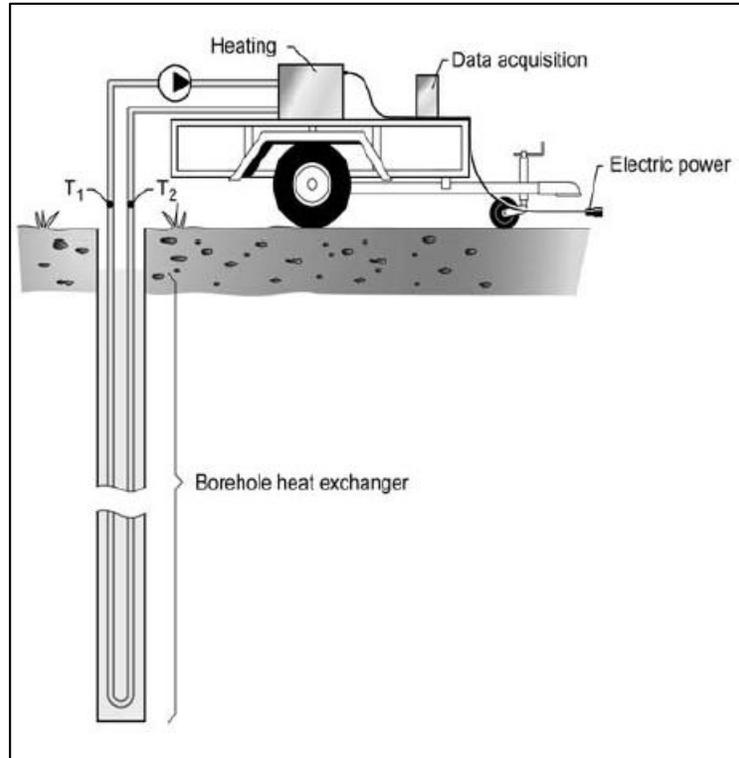
*Figure 2.2-6: Test setup for a TRT (Gehlin 2002).*
