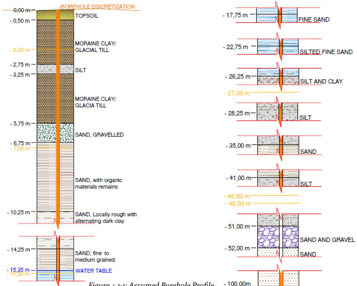
*Figure 4.1-1: Assumed Borehole Profile for the three boreholes studied.*
