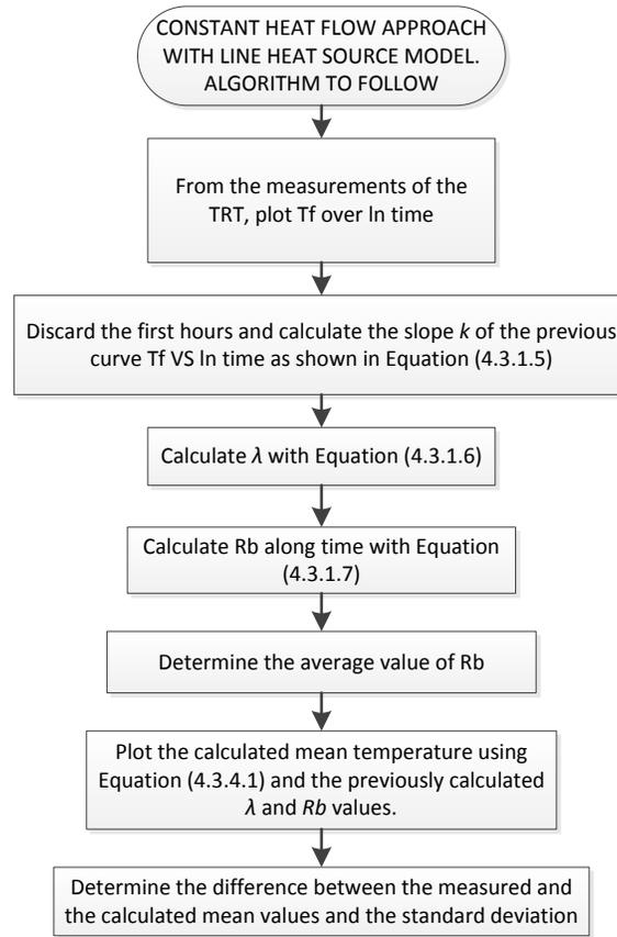
*Figure 4.3-2: Algorithm to follow for the evaluation of the data obtained the TRT.*
