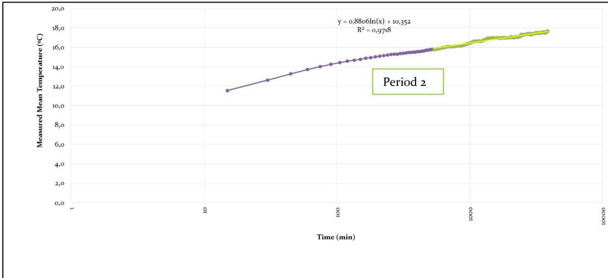
Figure 4.3-10: Measured mean temperature VS time logarithm and trend line for period 2 in Test 5.
