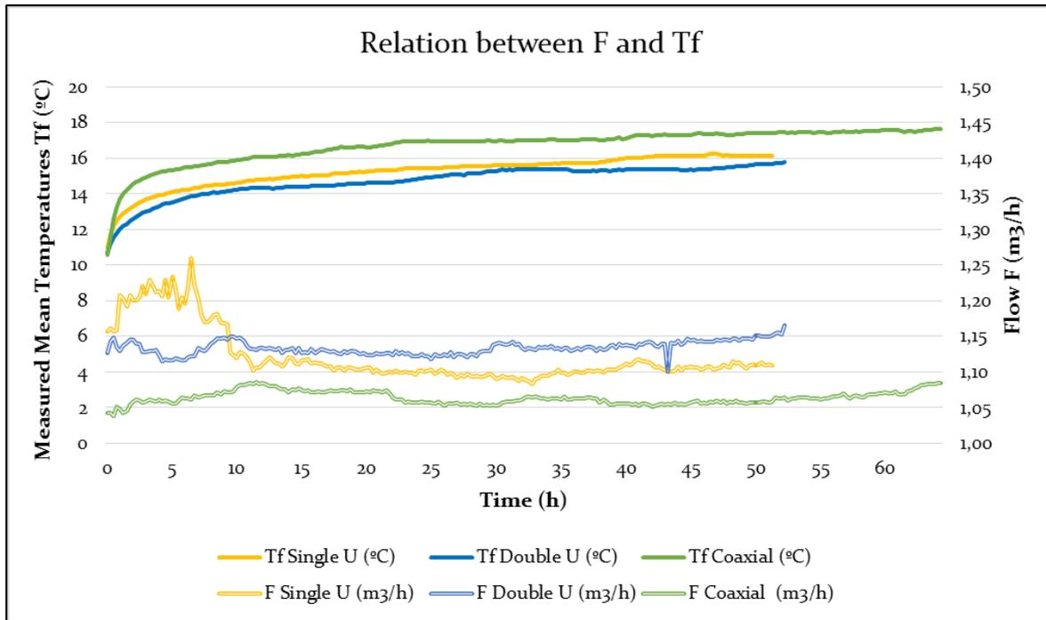
Figure 4.3-15: Graph showing the measured mean temperatures and the flow rate for the three tests.
