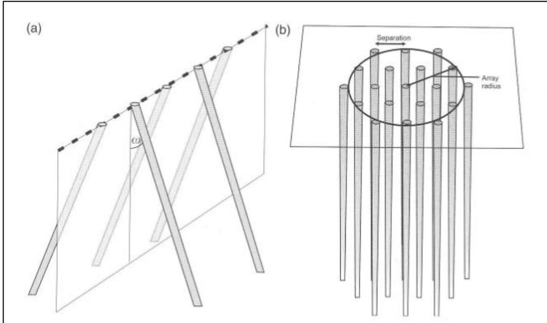
*Figure 2.2-4: a) Alternate inclined boreholes in opposing directions optimized for continuous heat extraction and rejection; b) Closed borehole array designed for BTES (Banks 2008).*
