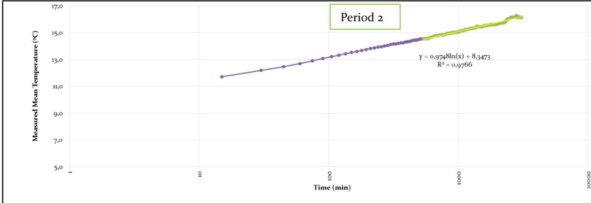
Figure 4.3-4: Measured mean temperature VS time logarithm and trend line for Period 2.
