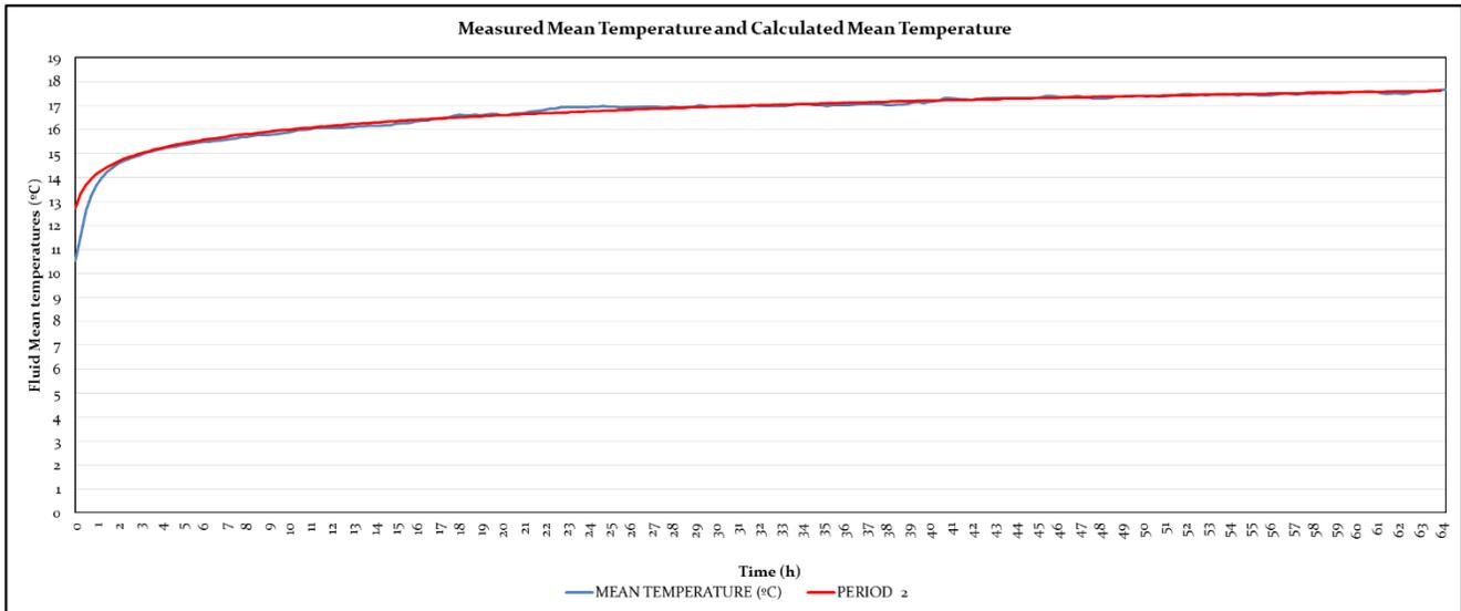
Figure 4.3-12: Fitting curve between measured meand temperature and the calculated one for period 2 in Test 5.
