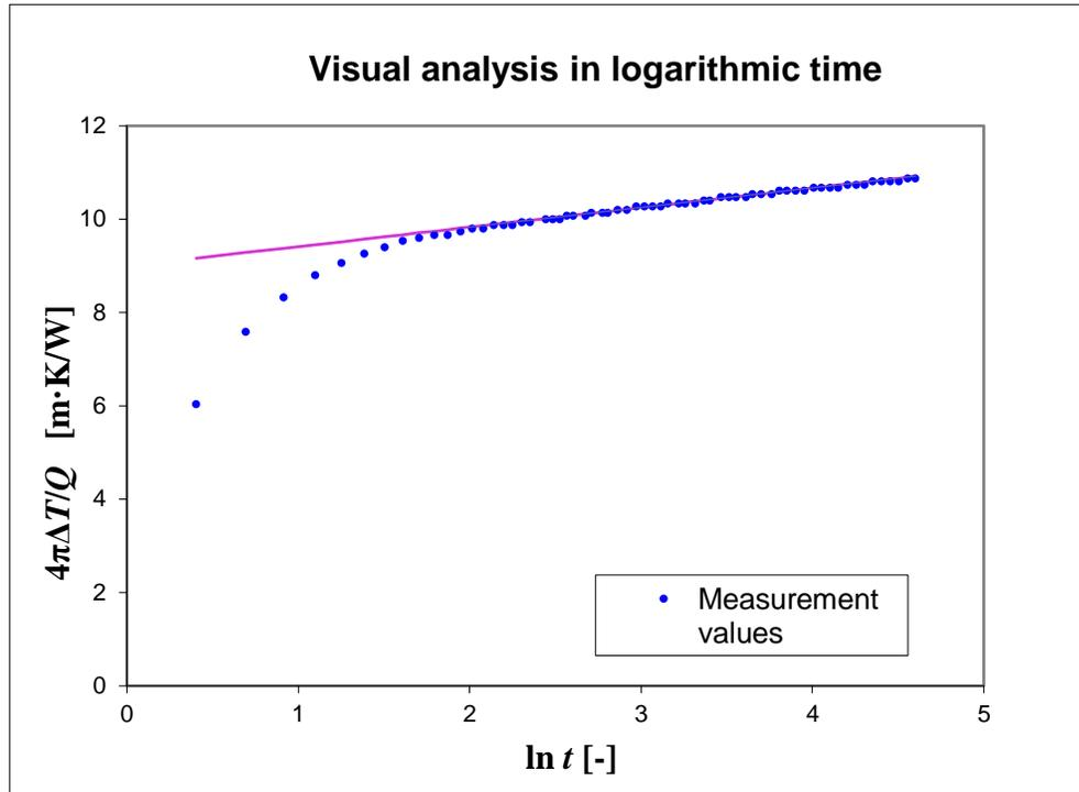
Figure 4.2-2: A typical plotting for  $4\pi\Delta T/Q$  vs time.
