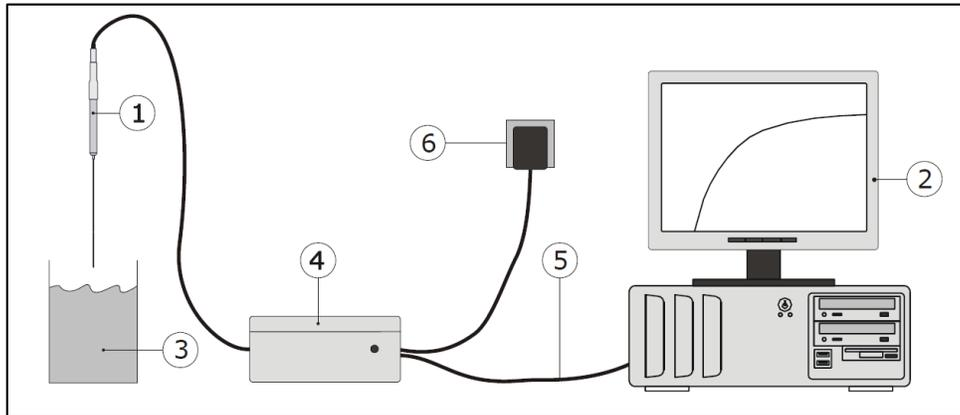
*Figure 4.2-1: Setup scheme for Hukseflux system TPSYSo2 (Hukseflux Thermal Sensors 2013b)*
